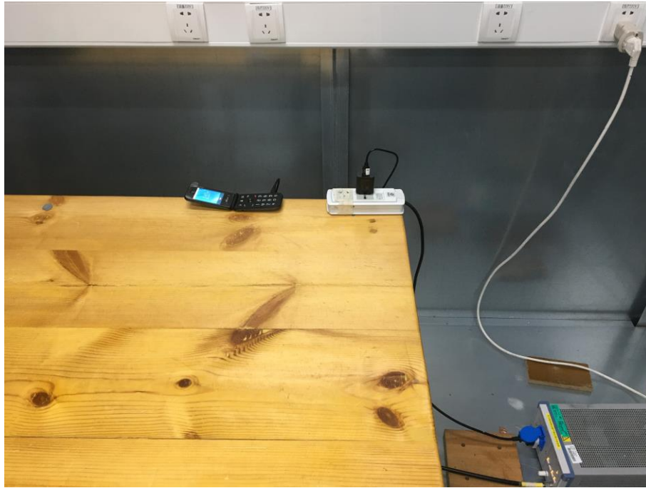
19. Conducted Emission (Part 15C, Bluetooth/Wi-Fi)
