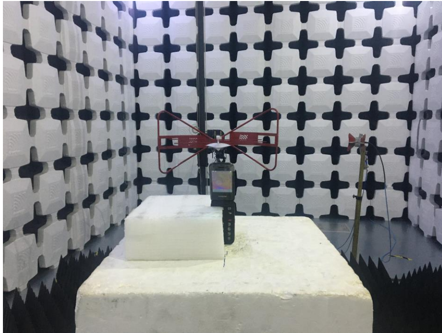
13. Radiated Emissions (Part 22/24/27/90,30MHz-18GHz)
