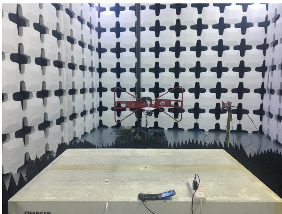
8. Radiated Emissions (Part 15B, FM receiver,1GHz-18GHz)
