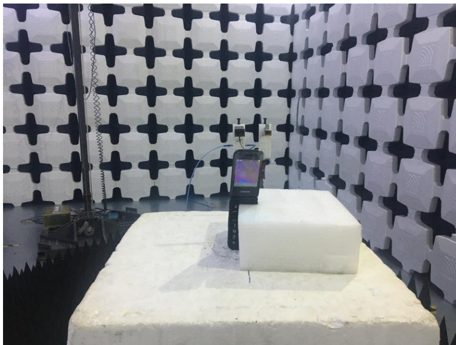
14. Radiated Emissions (Part 22/24/27/90, 18GHz -26.5GHz)
