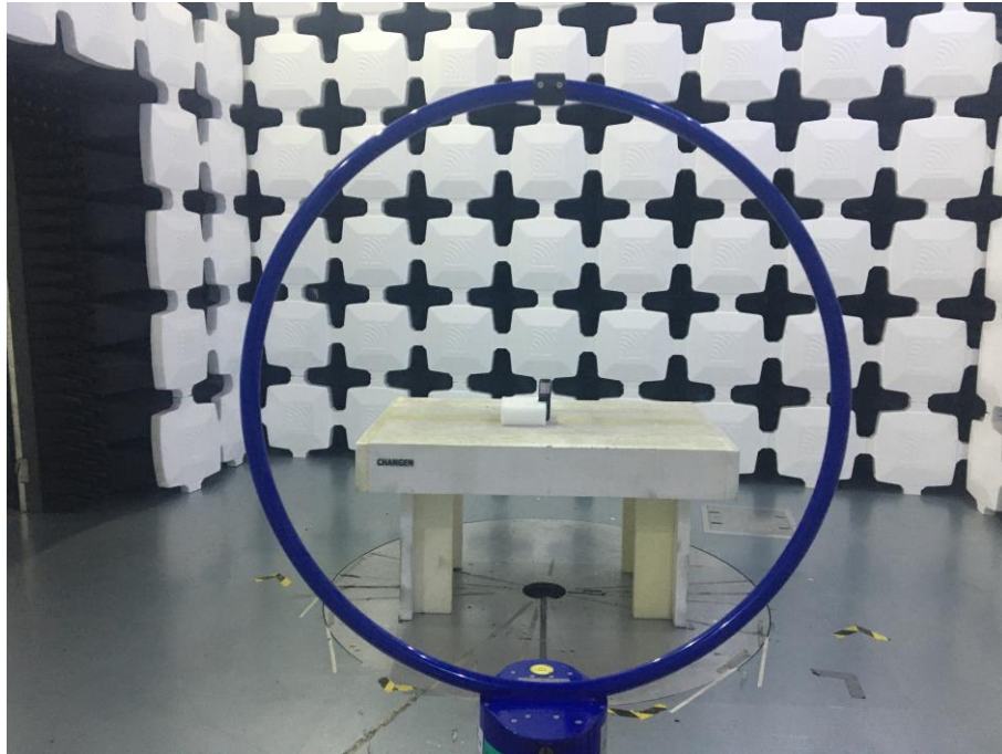
9. Radiated Emissions (Part 15C, 9kHz-30MHz)
