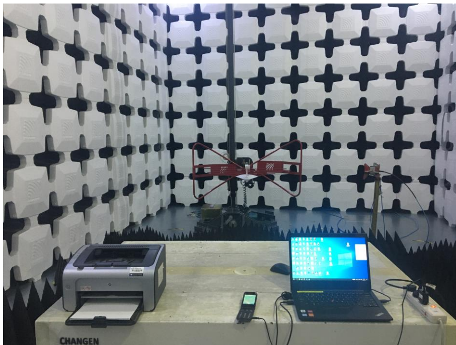
4. Radiated Emissions (Part 15B Bluetooth ,1GHz-18GHz)
