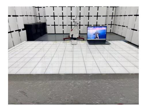
**Set-up for Radiated Spurious Emission, Above 1GHz**
