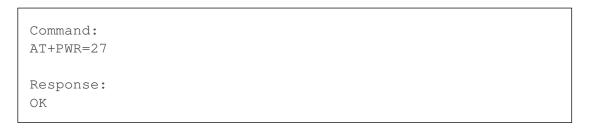
Besides setting a single output power for all antenna ports, you can also define separate output powers for each antenna by just adding more power parameters until you reach the number of antennas of your current setup. This includeds any connected multiplexer ports. Devices with only one antenna port and no outputs (DeskID UHF and QRG2) do not support multiple values for power.
