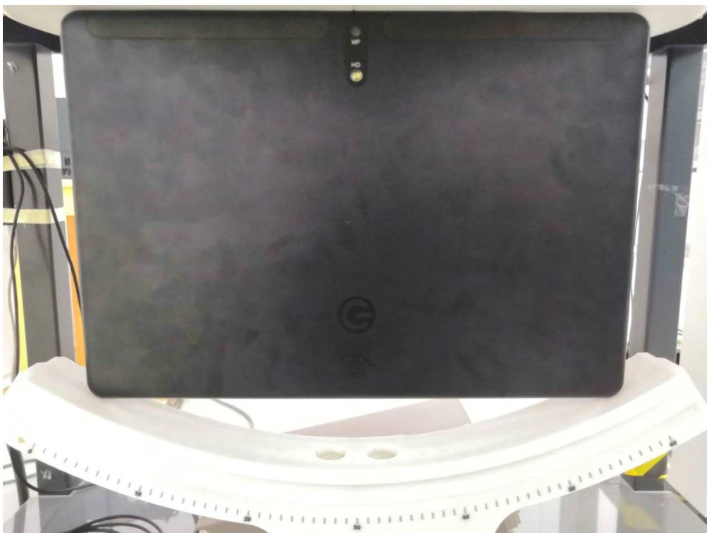
0mm body-worn Top Side Setup Photo (hotspot)
