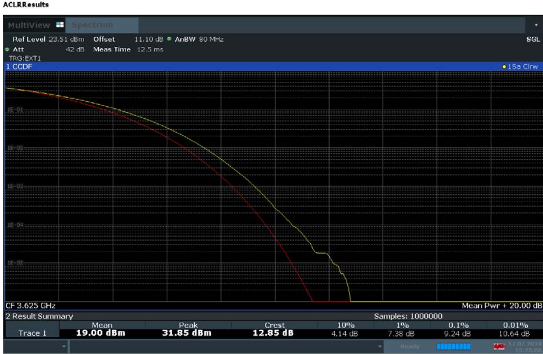
Plot 7-114. 16 User Beam PAR Plot (60.0MHz Total Bandwidth 64QAM - Mid Channel-SISO)
