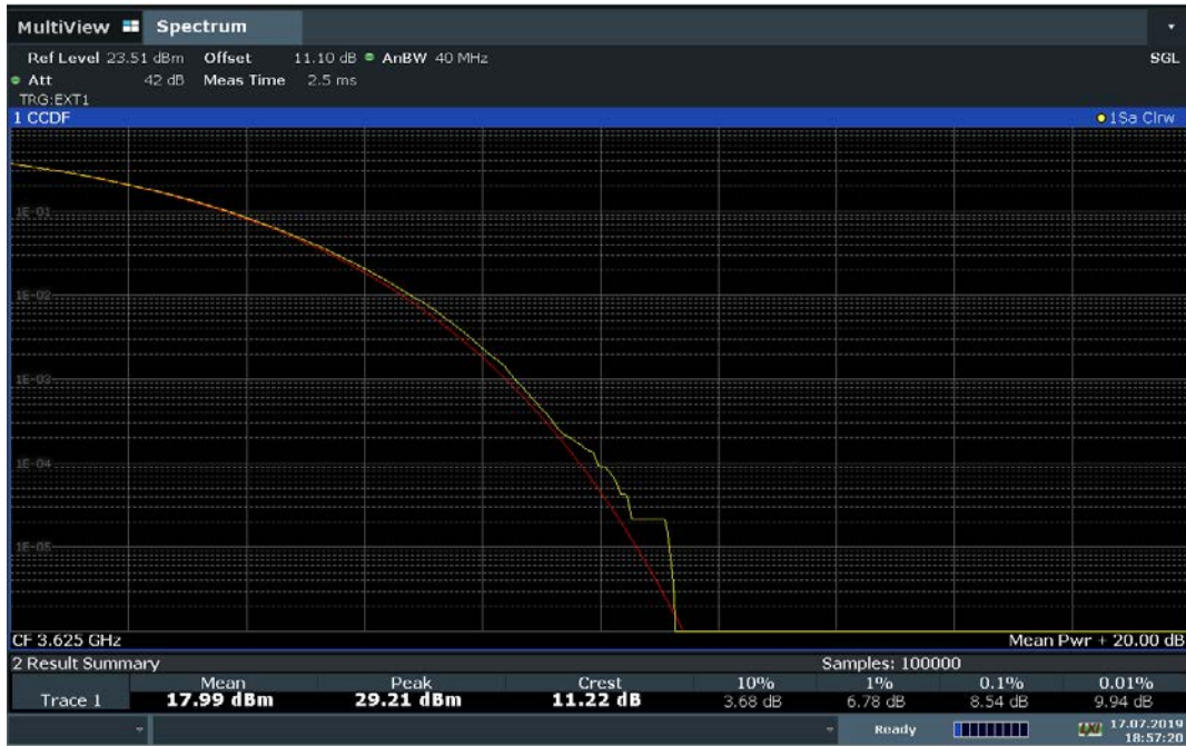
Plot 7-104. 16 User Beam PAR Plot (40.0MHz Total Bandwidth QPSK - Mid Channel-SISO)
