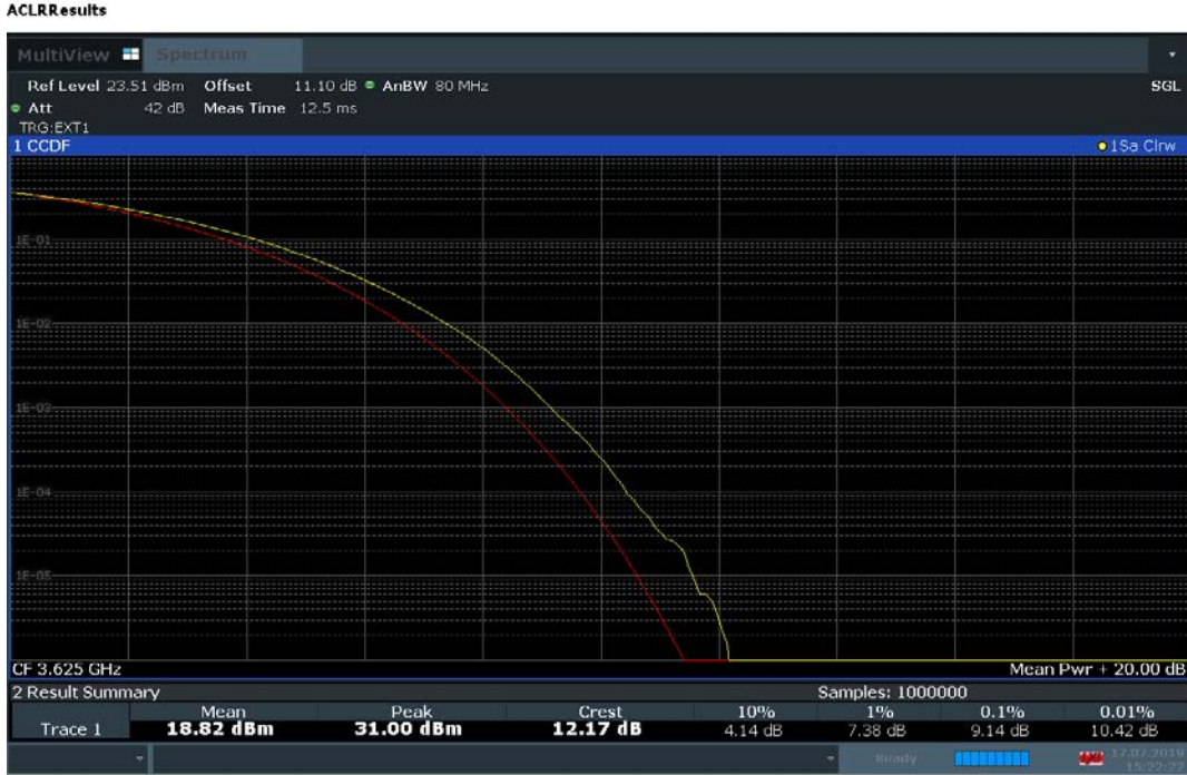
Plot 7-112. 16 User Beam PAR Plot (60.0MHz Total Bandwidth QPSK - Mid Channel-SISO)
