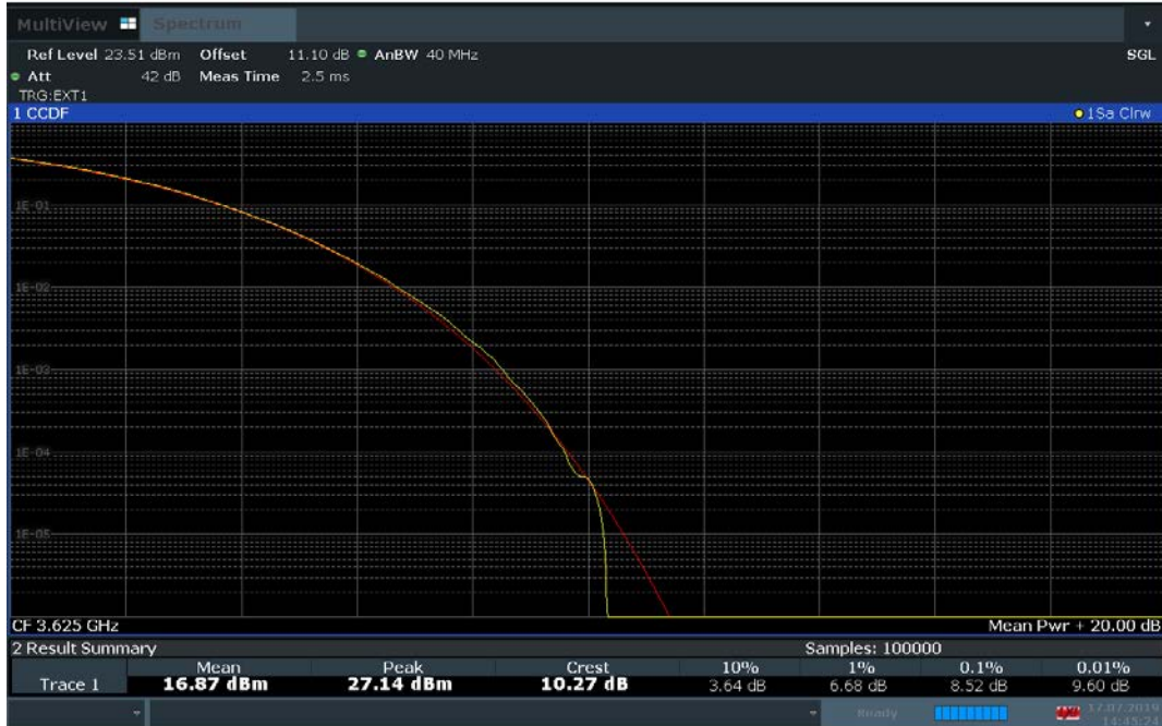
Plot 7-101. 16 User Beam PAR Plot (30.0MHz Total Bandwidth 16QAM - Mid Channel-SISO)
