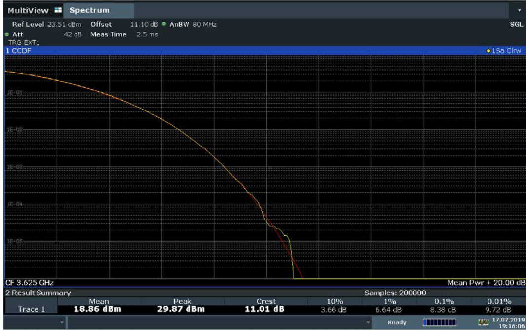
Plot 7-108. 16 User Beam PAR Plot (50.0MHz Total Bandwidth QPSK - Mid Channel-SISO)
