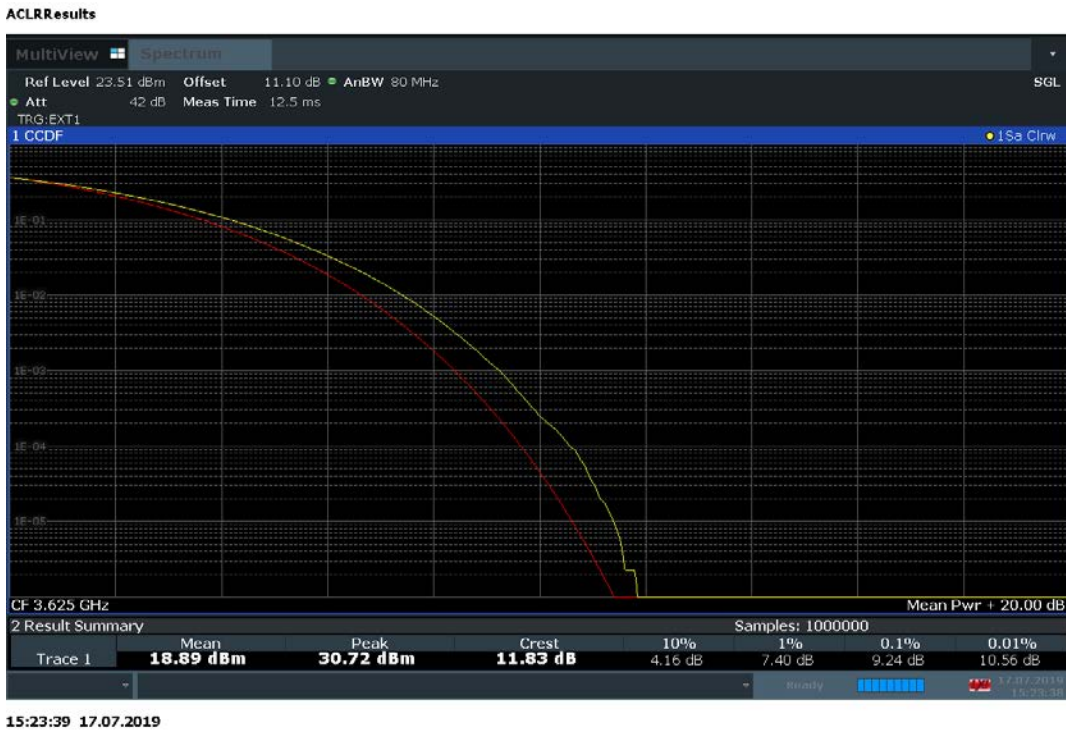
Plot 7-113. 16 User Beam PAR Plot (60.0MHz Total Bandwidth 16QAM - Mid Channel-SISO)
