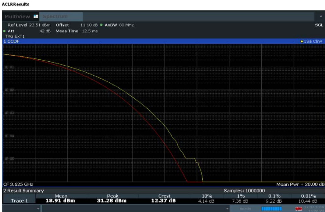
Plot 7-115. 16 User Beam PAR Plot (60.0MHz Total Bandwidth 256QAM - Mid Channel-SISO)
