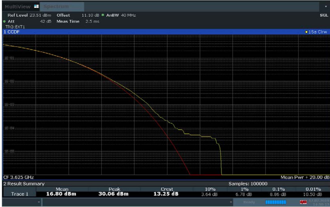
Plot 7-100. 16 User Beam PAR Plot (30.0MHz Total Bandwidth QPSK - Mid Channel-SISO)
