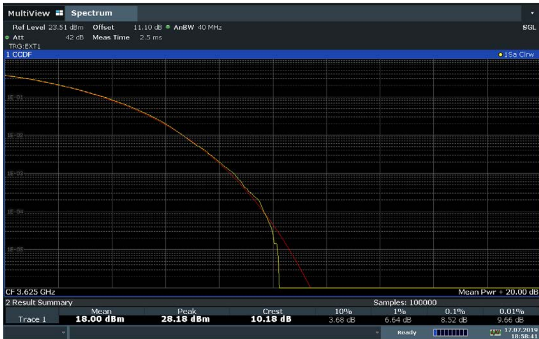
Plot 7-105. 16 User Beam PAR Plot (40.0MHz Total Bandwidth 16QAM - Mid Channel-SISO)
