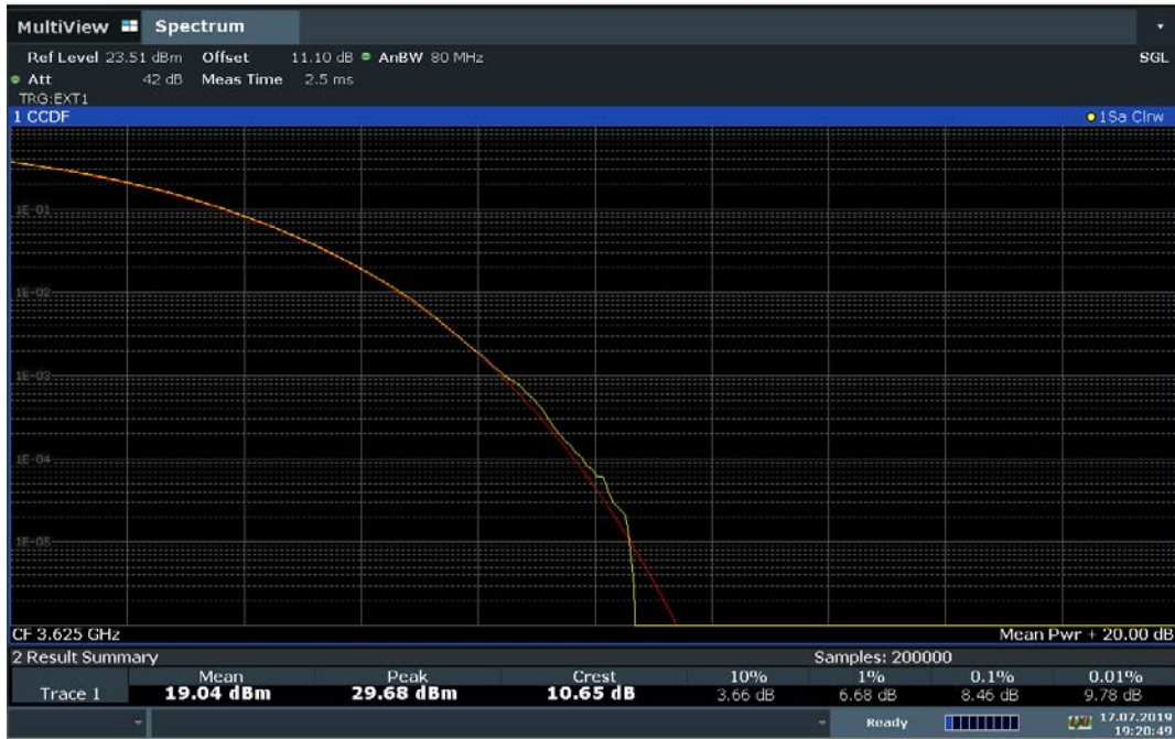
Plot 7-110. 16 User Beam PAR Plot (50.0MHz Total Bandwidth 64QAM - Mid Channel-SISO)
