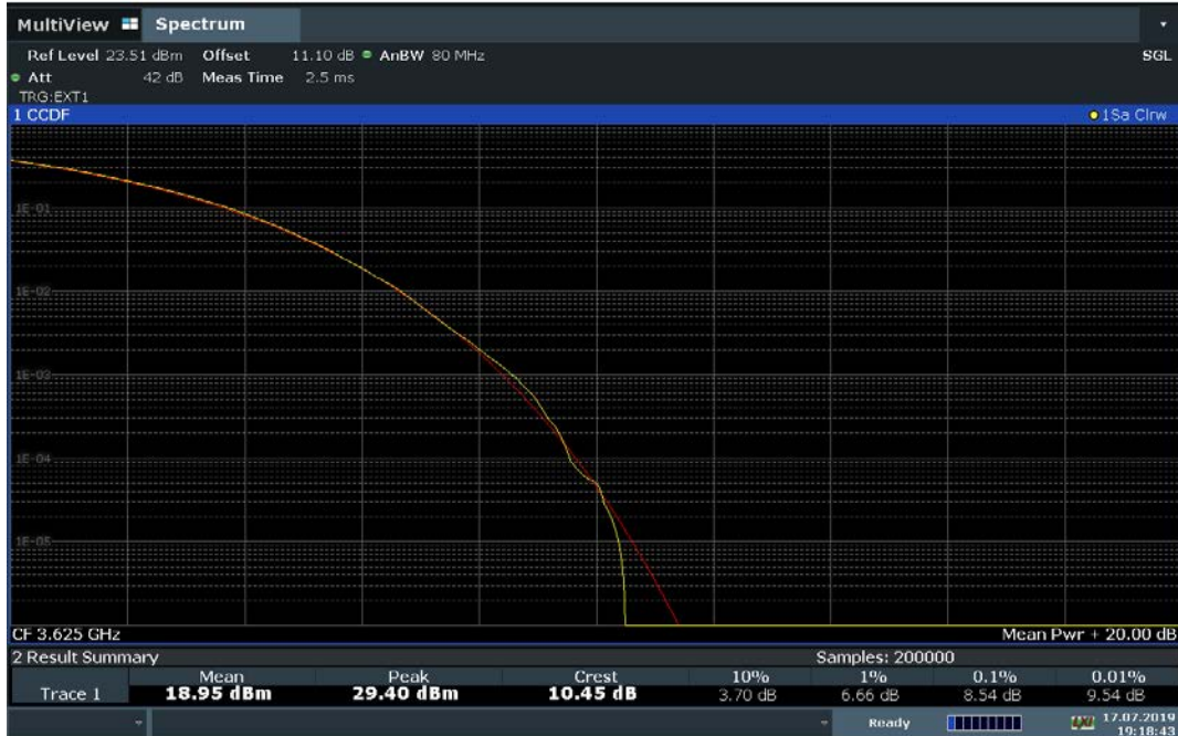
Plot 7-109. 16 User Beam PAR Plot (50.0MHz Total Bandwidth 16QAM - Mid Channel-SISO)
