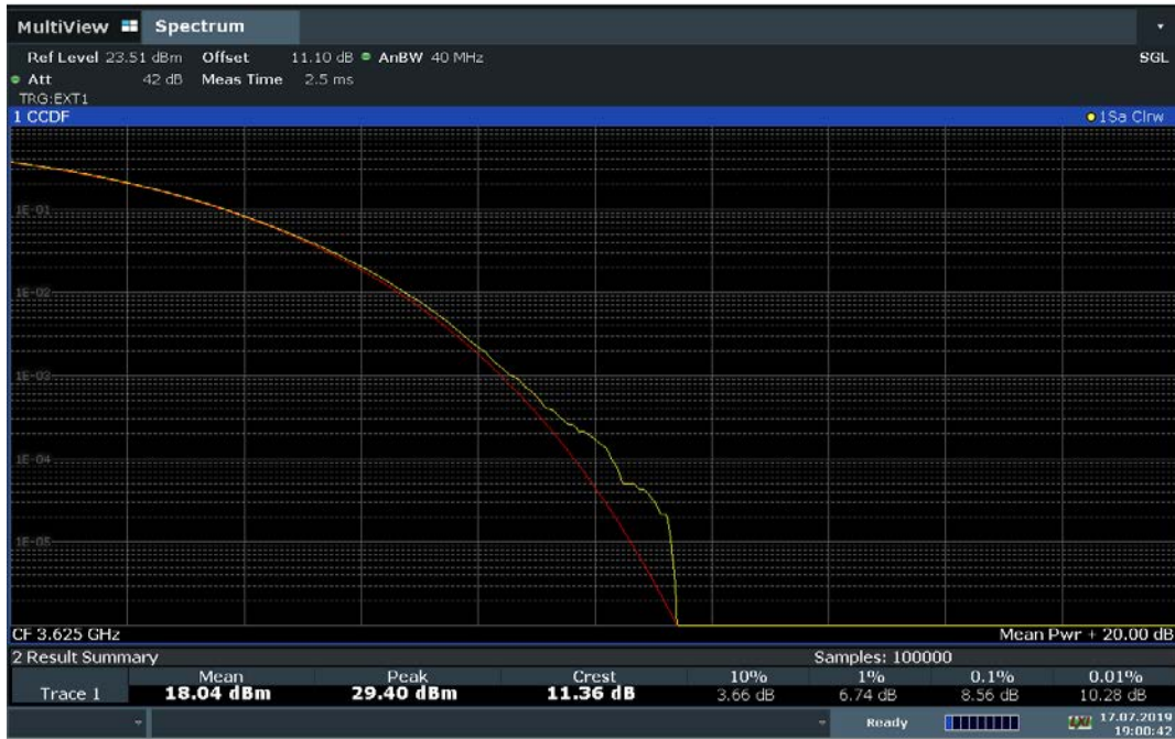
Plot 7-106. 16 User Beam PAR Plot (40.0MHz Total Bandwidth 64QAM - Mid Channel-SISO)
