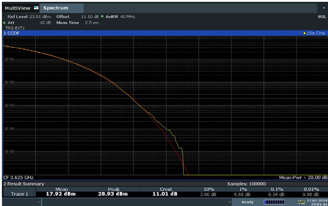
Plot 7-107. 16 User Beam PAR Plot (40.0MHz Total Bandwidth 256QAM - Mid Channel-SISO)
