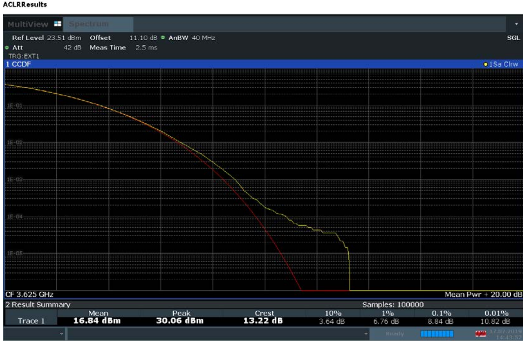
Plot 7-102. 16 User Beam PAR Plot (30.0MHz Total Bandwidth 64QAM - Mid Channel-SISO)
