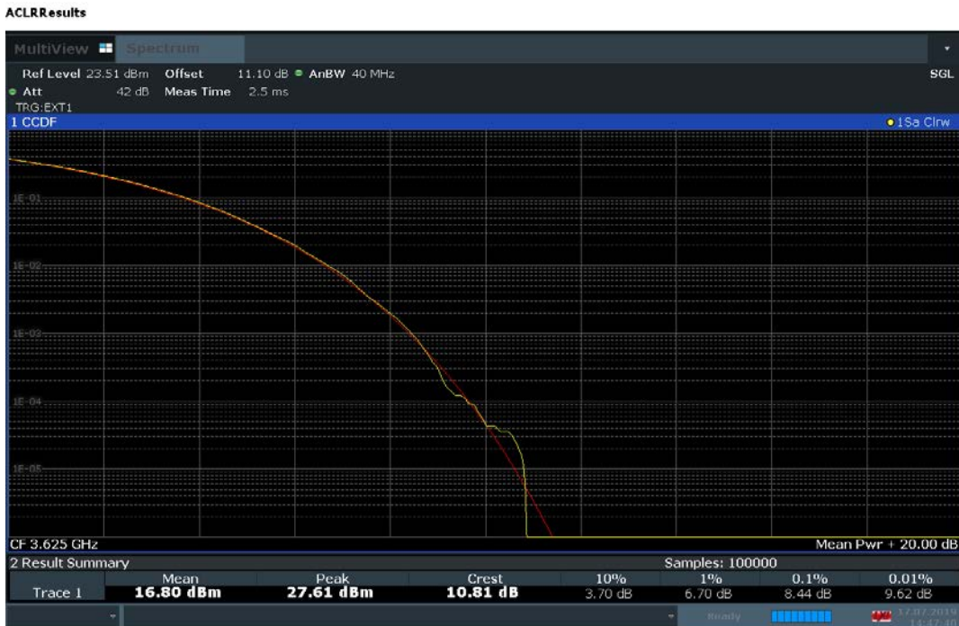
Plot 7-103. 16 User Beam PAR Plot (30.0MHz Total Bandwidth 256QAM - Mid Channel-SISO)
