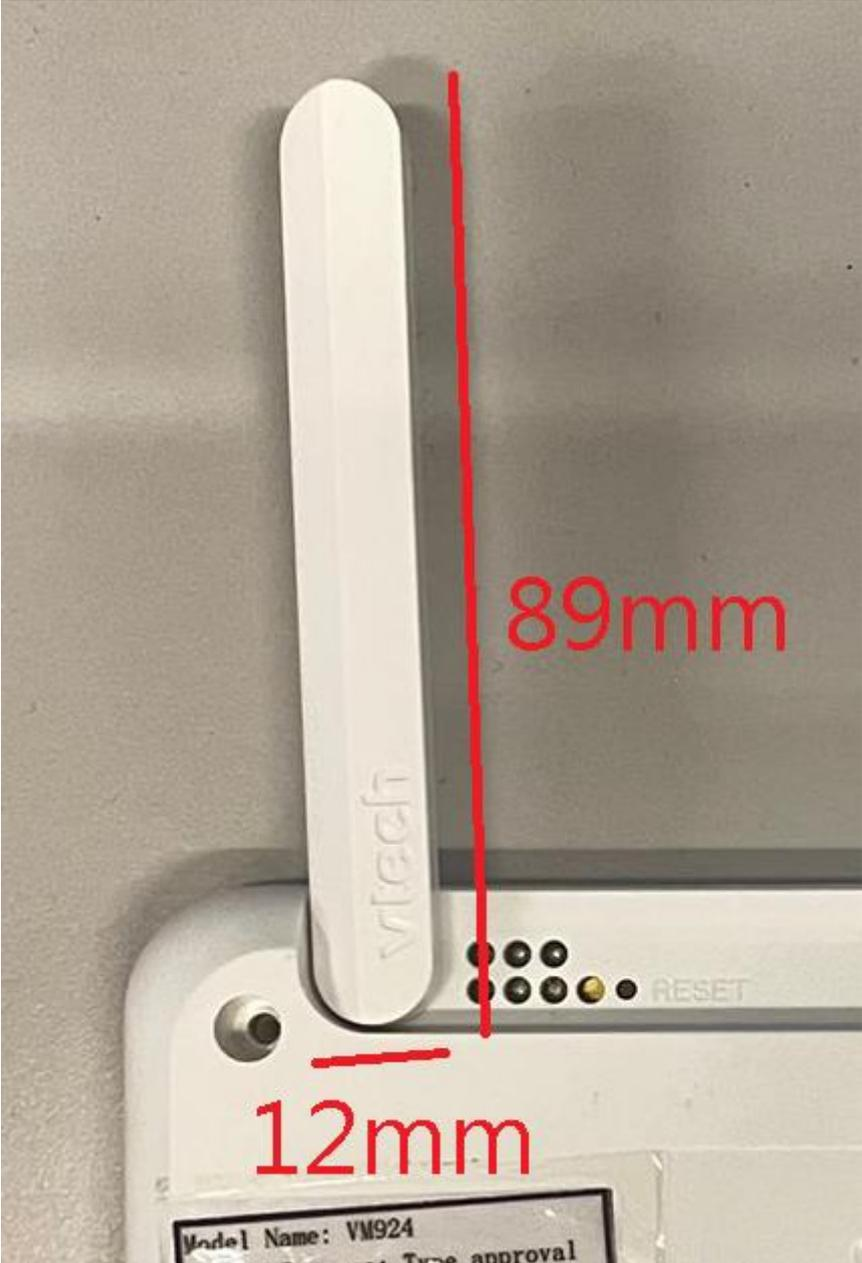
Figure 1 Physical dimension (mm)
