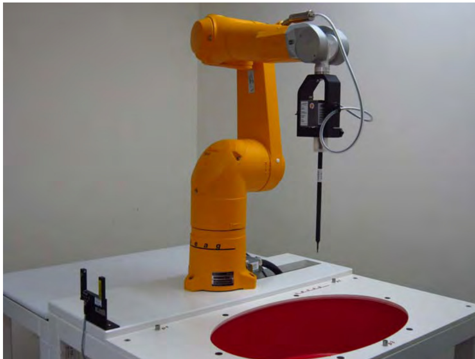
Fig.1 Photograph of the SAR measurement system
