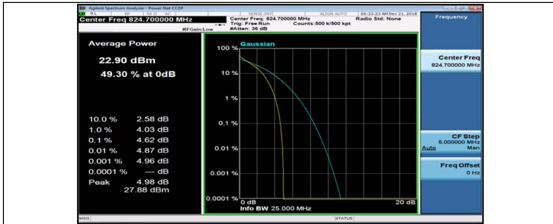
(Channel Bandwidth: 1.4 MHz)_MCH_QPSK_1RB#0
