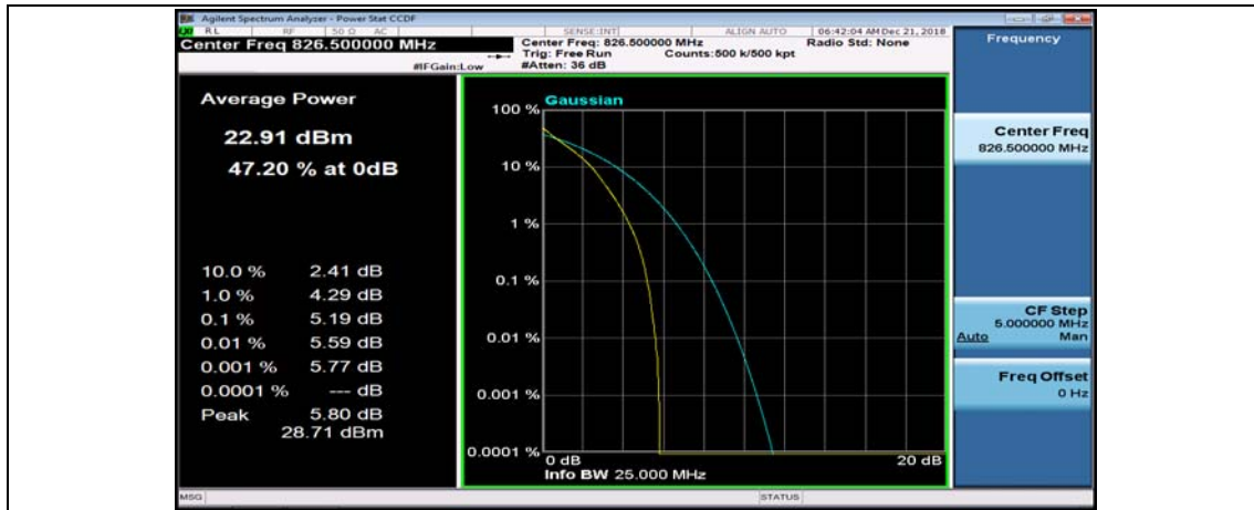
(Channel Bandwidth: 5 MHz)_MCH_QPSK_1RB#0
