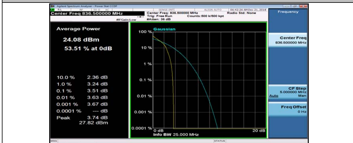
(Channel Bandwidth: 5 MHz)_MCH_QPSK_1RB#24
