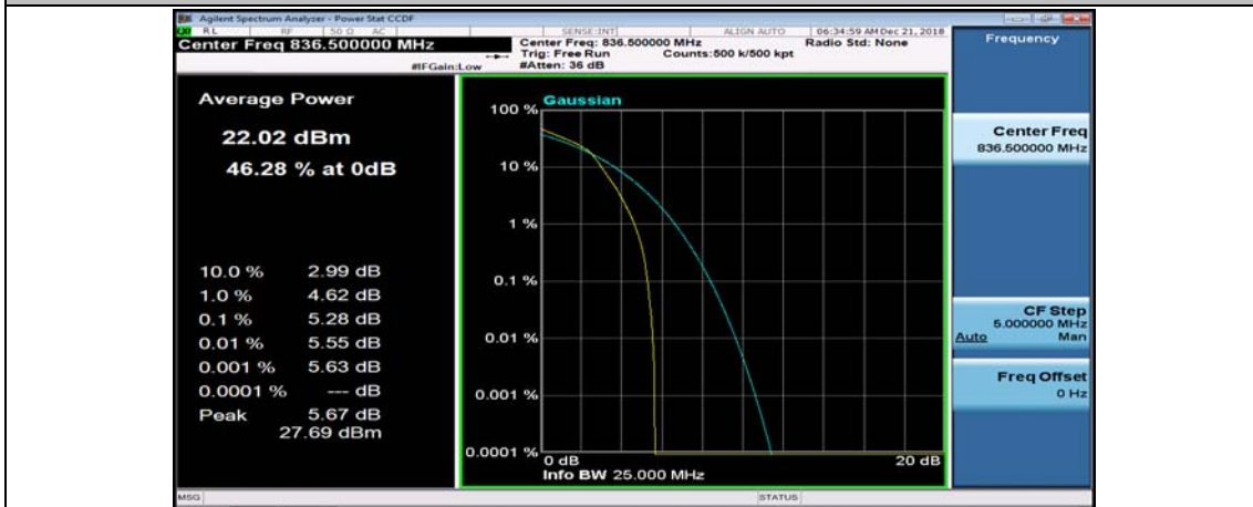
(Channel Bandwidth: 1.4 MHz)_MCH_16QAM_6RB#0
