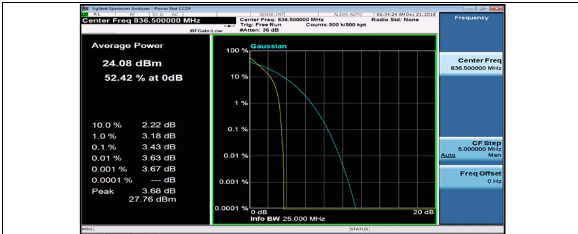
(Channel Bandwidth: 1.4 MHz)_MCH_QPSK_6RB#0
