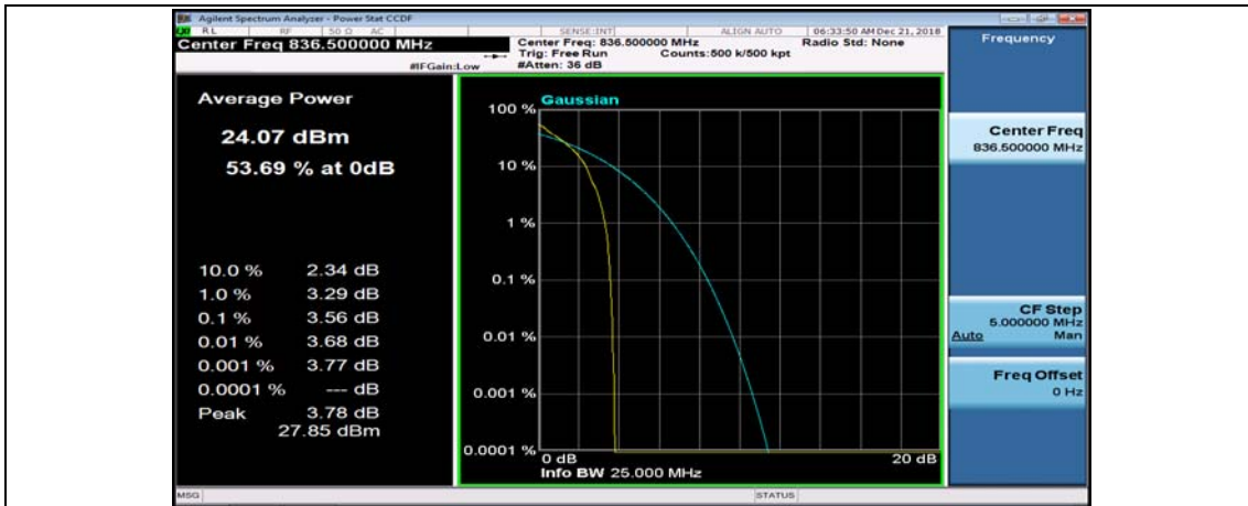
(Channel Bandwidth: 1.4 MHz)_MCH_QPSK_3RB#0
