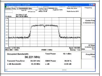
Mode:802.11ac VHT40 Frequency:5755MHz
