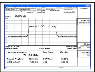
Mode:802.11ac VHT80 Frequency:5775MHz
