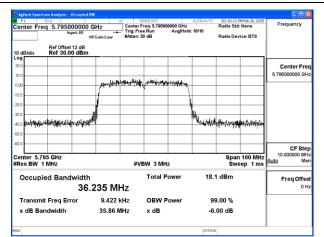
Mode:802.11ac VHT40 Frequency:5755MHz
