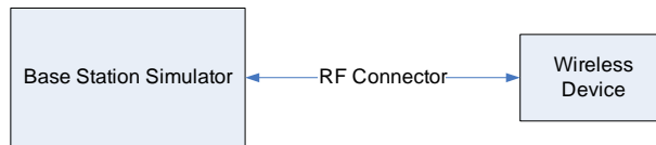
Figure 9-1 Power Measurement Setup
