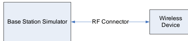
Figure 9-2 Power Measurement Setup
