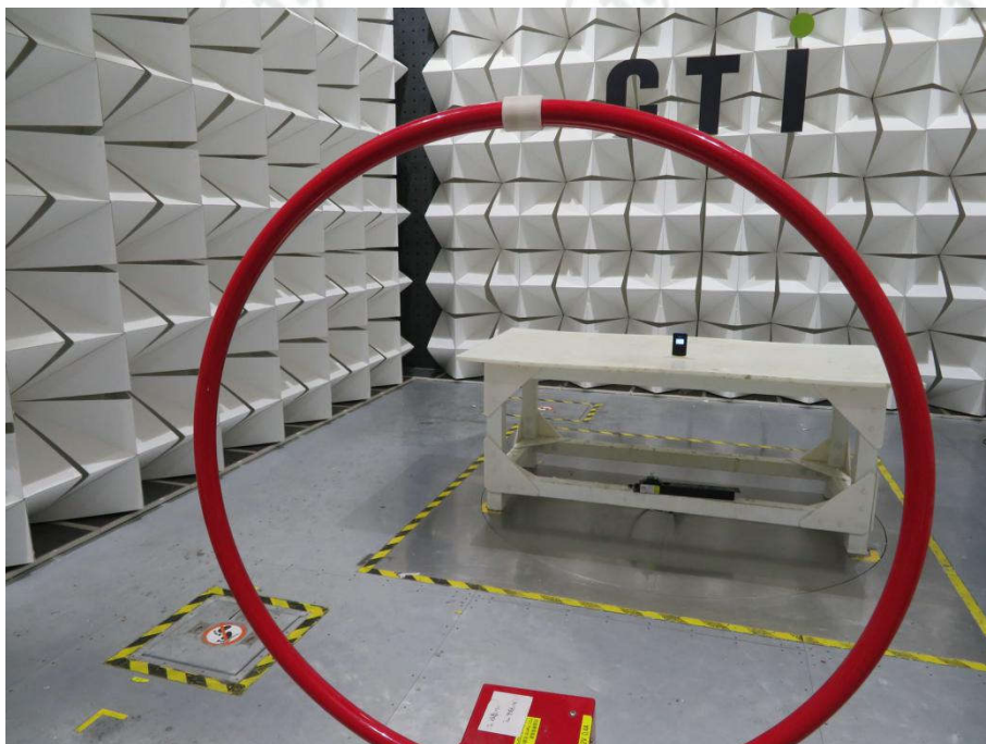
Radiated emission Test Setup-1 (9kHz~30MHz)
