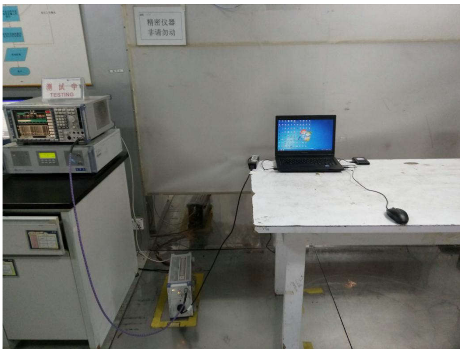
Conducted Emissions Test Setup
