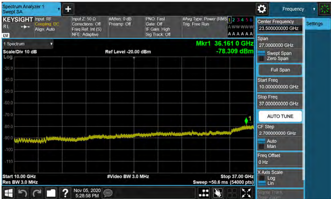
BAND 48. Conducted Spurious Plot 2 (10 MHz Ch. 56690 QPSK RB 1, Offset 0)
