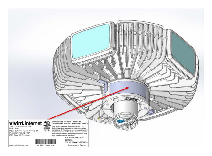
Note: The artwork is thermally printed black on white or silver outdoor rated label material. A high-tack outdoor rated adhesive backing permanently secures the label to the device at the location shown above.
