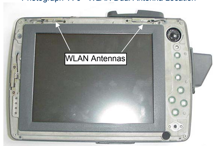
Photograph A-6 - WLAN Dual Antenna Location
