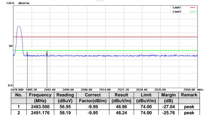
Note: GFSK,  $\pi/4$ -DQPSK, 8DPSK of the nohopping and hopping mode all have been test, the worst case is GFSK of the nohopping mode, this report only show the worst case.
