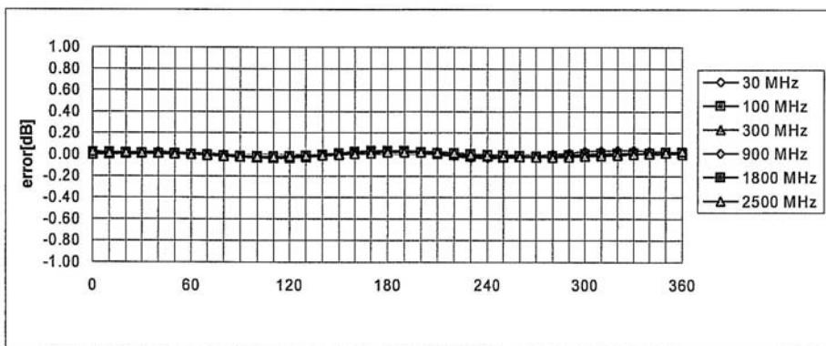
**Axial Isotropy Error  $< \pm 0.2$  dB**
