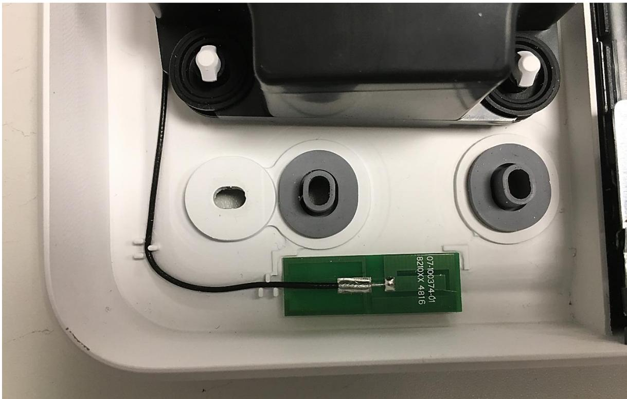
Antenna in the corner of the product. Rear side of the antenna PCB is only glue, no PCB traces.
