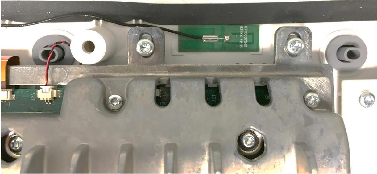
Antenna is near top center of the product. The rear side of the antenna PCB is only glue, no PCB traces.
