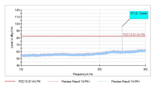
The peak above the limit is the carrier frequency Bluetooth Low Energy (2440 MHz).
