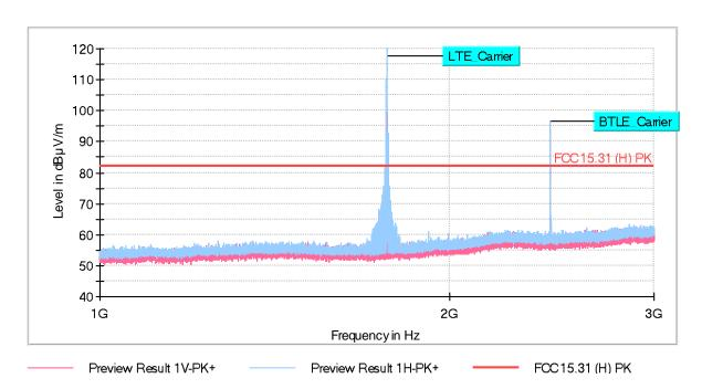
The peak above the limit is the carrier frequency LTE Cat-M1 Band 66 (1770 MHz).
