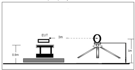
(B) Radiated Emission Test-Up Frequency 30MHz~1GHz
