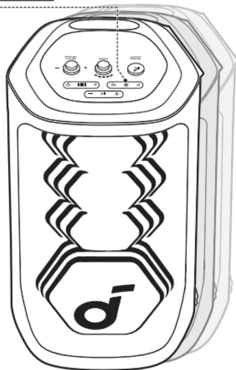
**With one speaker connected to a smartphone, press the AuraCast button on up to 100 soundcore speakers with AuraCast function to synchronize audio and light.**
