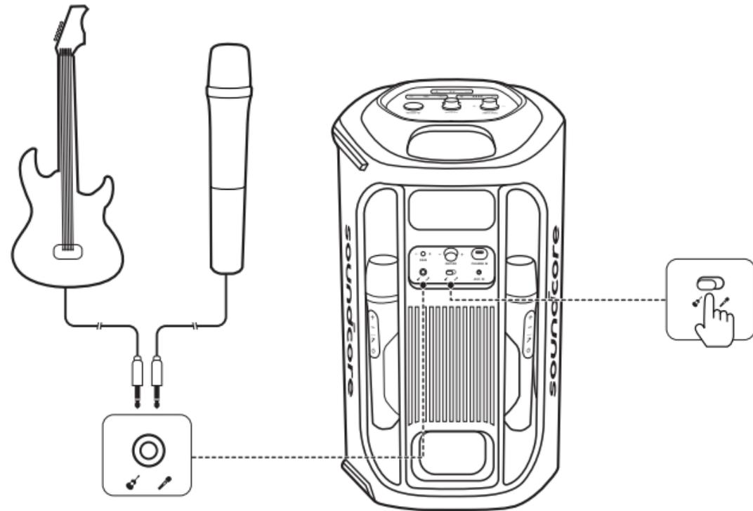
**Connect a microphone or guitar to the speaker through 6.5mm audio cables (not supplied).**
