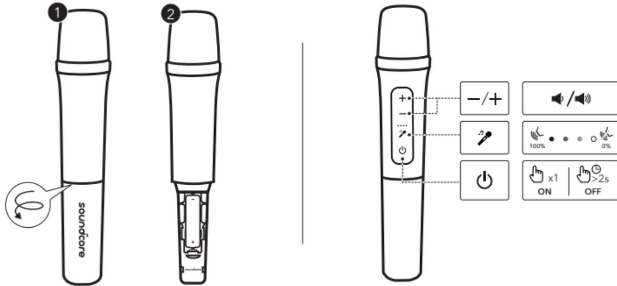
**For first-time use of the wireless microphone, unscrew battery cover and install two AA batteries. Once you power on the wireless microphone, it will automatically connect to the speaker. Through the physical buttons on the microphone, you can adjust its volume and the level of the original vocals being removed in karaoke.**
