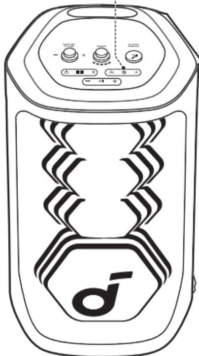
**With one speaker connected to a smartphone, press the AuraCast button simultaneously on both speakers to enter TWS pairing mode. Upon successful pairing, you will hear a sound prompt. Then double press the AuraCast button on either speaker to assign the left and right audio channels.**
