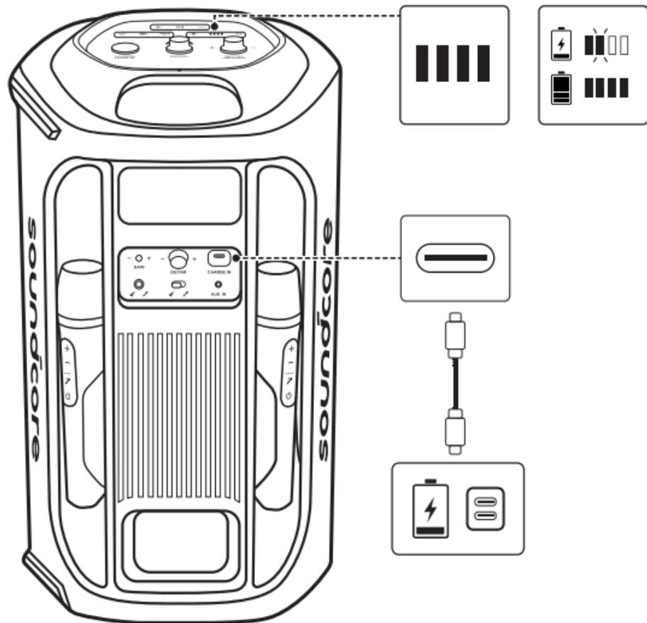
**Connect the speaker to the power source with a C-C cable.**
