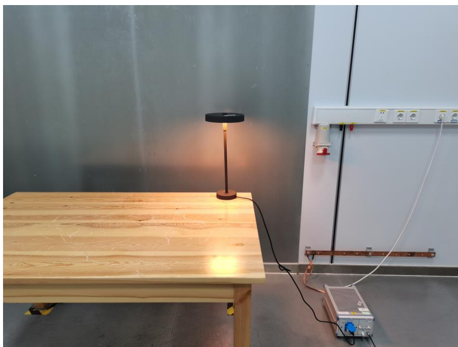
Fig. 4 Power line conducted emission setup photo
