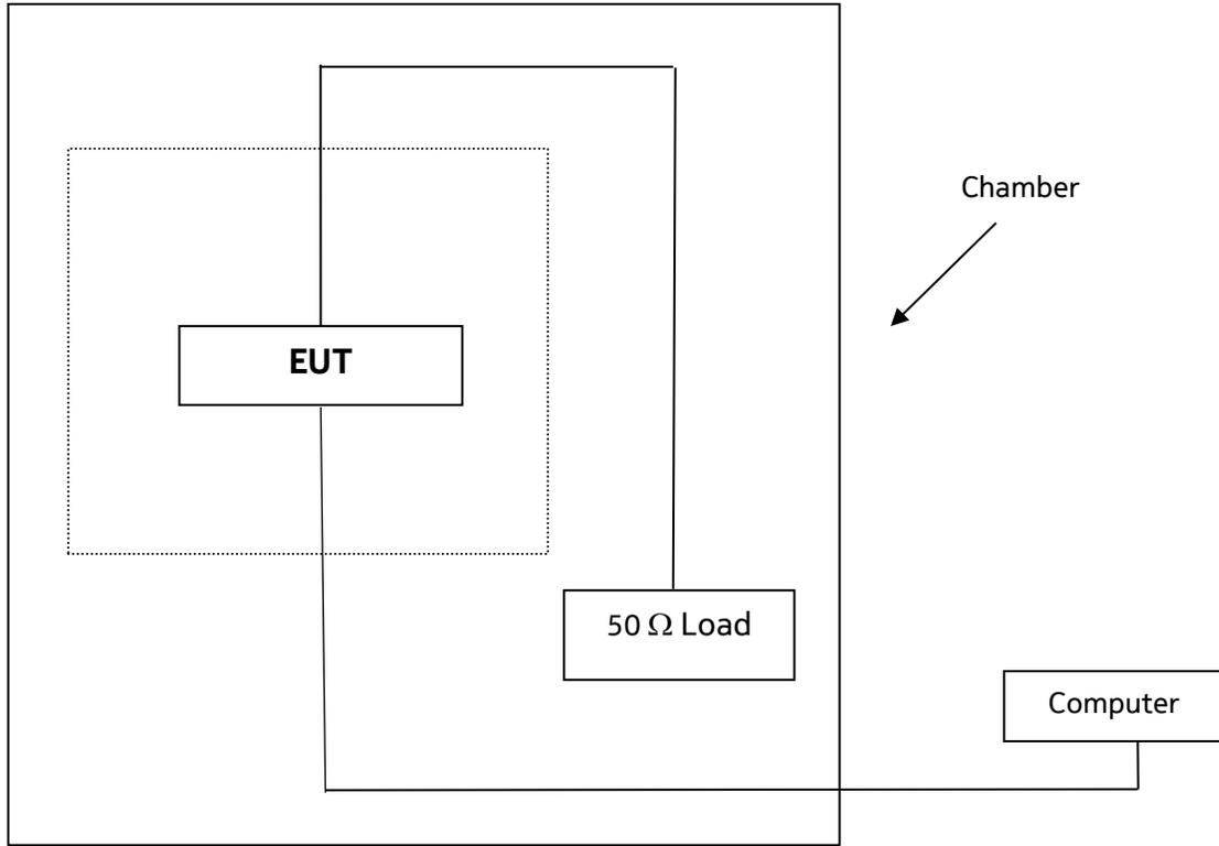
Figure 2. Setup Diagram of Radiated Test
