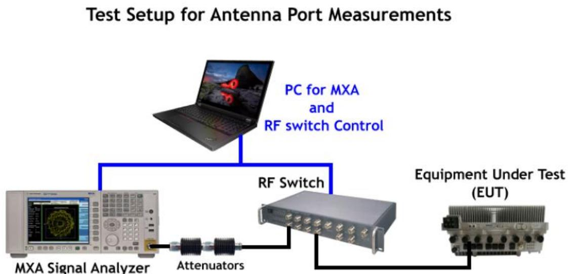
**Figure 1. Setup Diagram of Conducted Test for Measurement at Antenna Ports.**
