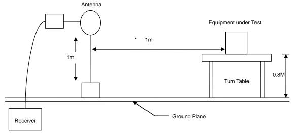
30MHz- 1GHz Test Setup
