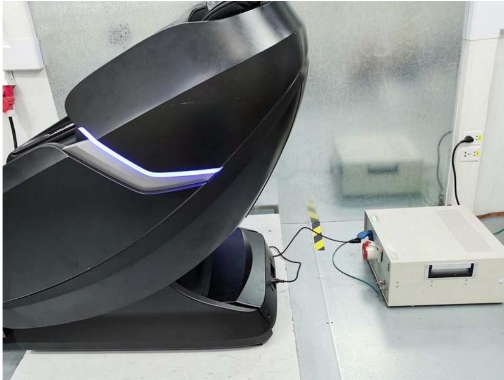
Conducted Emission Test Setup:
