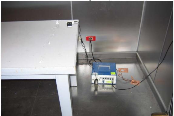
**Conducted Emission Set up Photo (Audio-in Mode)**
