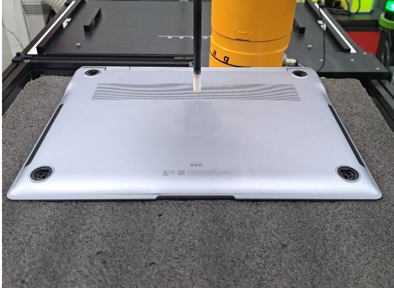
Test Setup Photo 3 - Near Field Power Density, Bottom Edge at 10.02 mm
