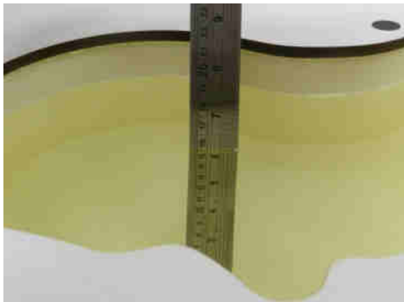
Fig 10.1 Photo of Liquid Height for Head SAR
