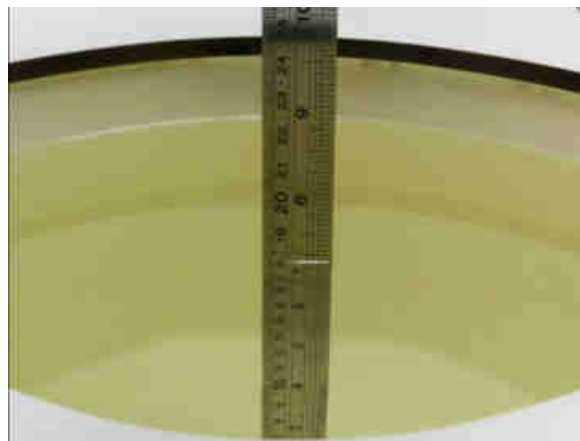
Fig 10.2 Photo of Liquid Height for Body SAR
