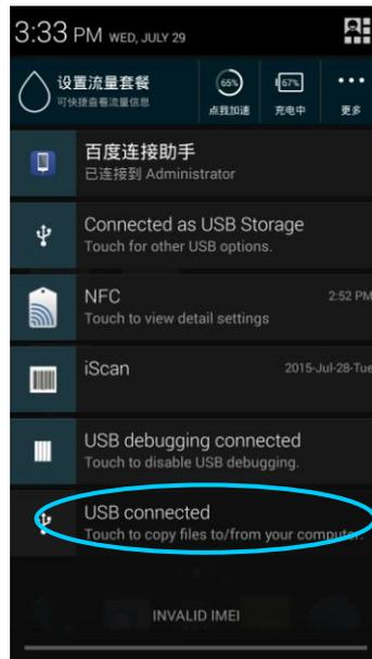
Click the option to open the USB storage device and copy files between the PC and the device
