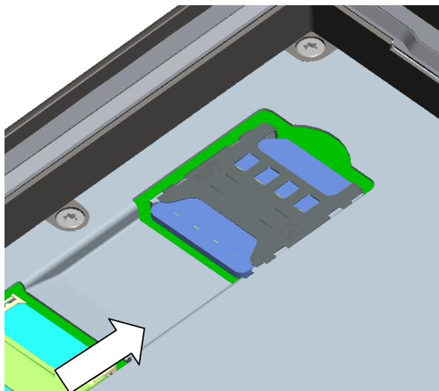
Figure 1-4 Inserting a SIM card
