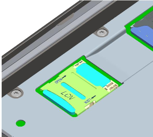
Figure 1-3 Inserting an SD card
