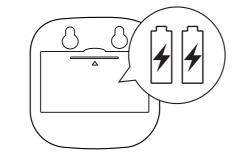
Remove the battery cover by gently pressing down on the tab. Insert the two AA batteries and reattach battery cover.
