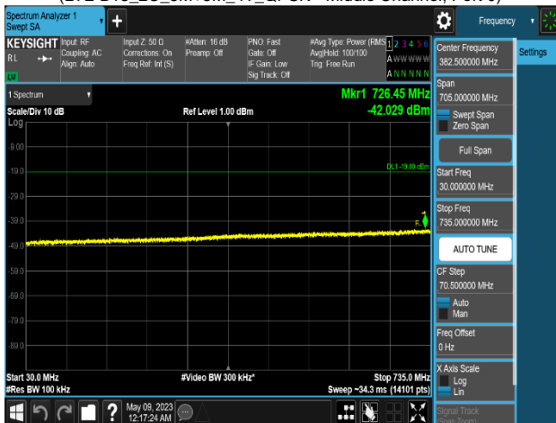
Plot 8-780. Conducted Spurious Emission Plot 30 MHz to 735 MHz (LTE B13_2C_5M+5M_4T_QPSK - Middle Channel, Port 0)
