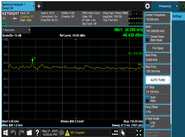
Plot 8-796. Conducted Spurious Emission Plot 9 kHz to 150 kHz (Multi-Band_LTE B13_1C_10M+NB-IoT(2GB)+LTE B5_1C_10M _4T_QPSK-Middle+Low Channel, Port 3)
