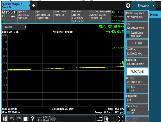
Plot 8-792. Conducted Spurious Emission Plot 30 MHz to 735 MHz (LTE B13_1C_10M+NB-IoT(2GB)_4T_QPSK-Mid Channel, Port 0)
