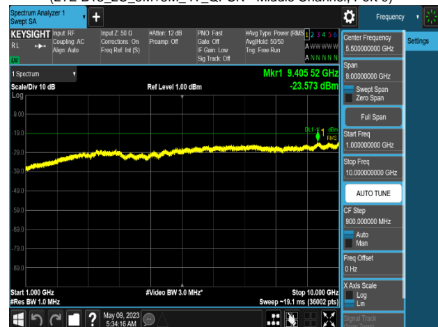
Plot 8-783. Conducted Spurious Emission Plot 1 GHz to 10 GHz (LTE B13_2C_5M+5M_4T_QPSK - Middle Channel, Port 0)
