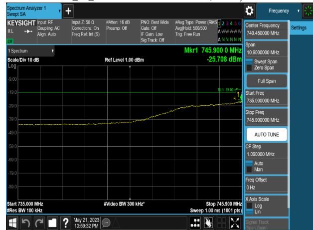
Plot 8-799. Conducted Spurious Emission Plot 735 MHz to 745.9 MHz (Multi-Band_LTE B13_1C_10M+NB-IoT(2GB)+LTE B5_1C_10M _4T_QPSK-Middle+Low Channel, Port 3)
