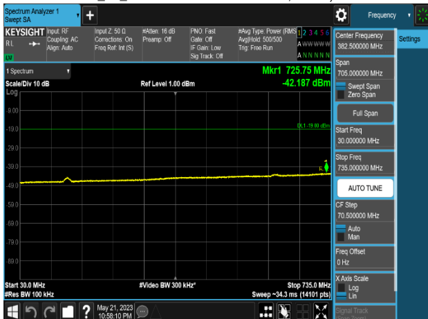
Plot 8-798. Conducted Spurious Emission Plot 30 MHz to 735 MHz (Multi-Band_LTE B13_1C_10M+NB-IoT(2GB)+LTE B5_1C_10M _4T_QPSK-Middle+Low Channel, Port 3)
