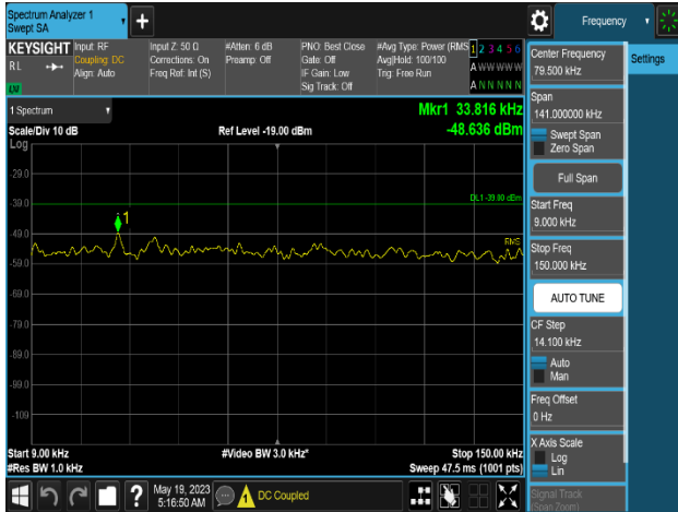
Plot 8-790. Conducted Spurious Emission Plot 9 kHz to 150 kHz (LTE B13_1C_10M+NB-IoT(2GB)_4T_QPSK-Mid Channel, Port 0)
