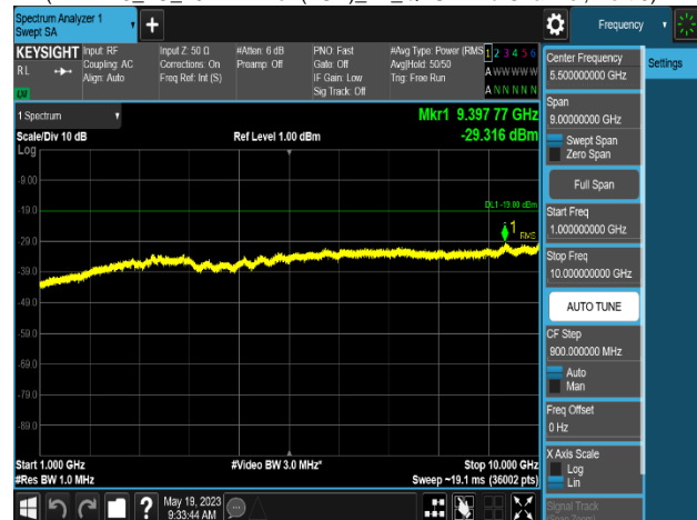
Plot 8-795. Conducted Spurious Emission Plot 1 GHz to 10 GHz (LTE B13_1C_10M+NB-IoT(2GB)_4T_QPSK-Mid Channel, Port 0)
