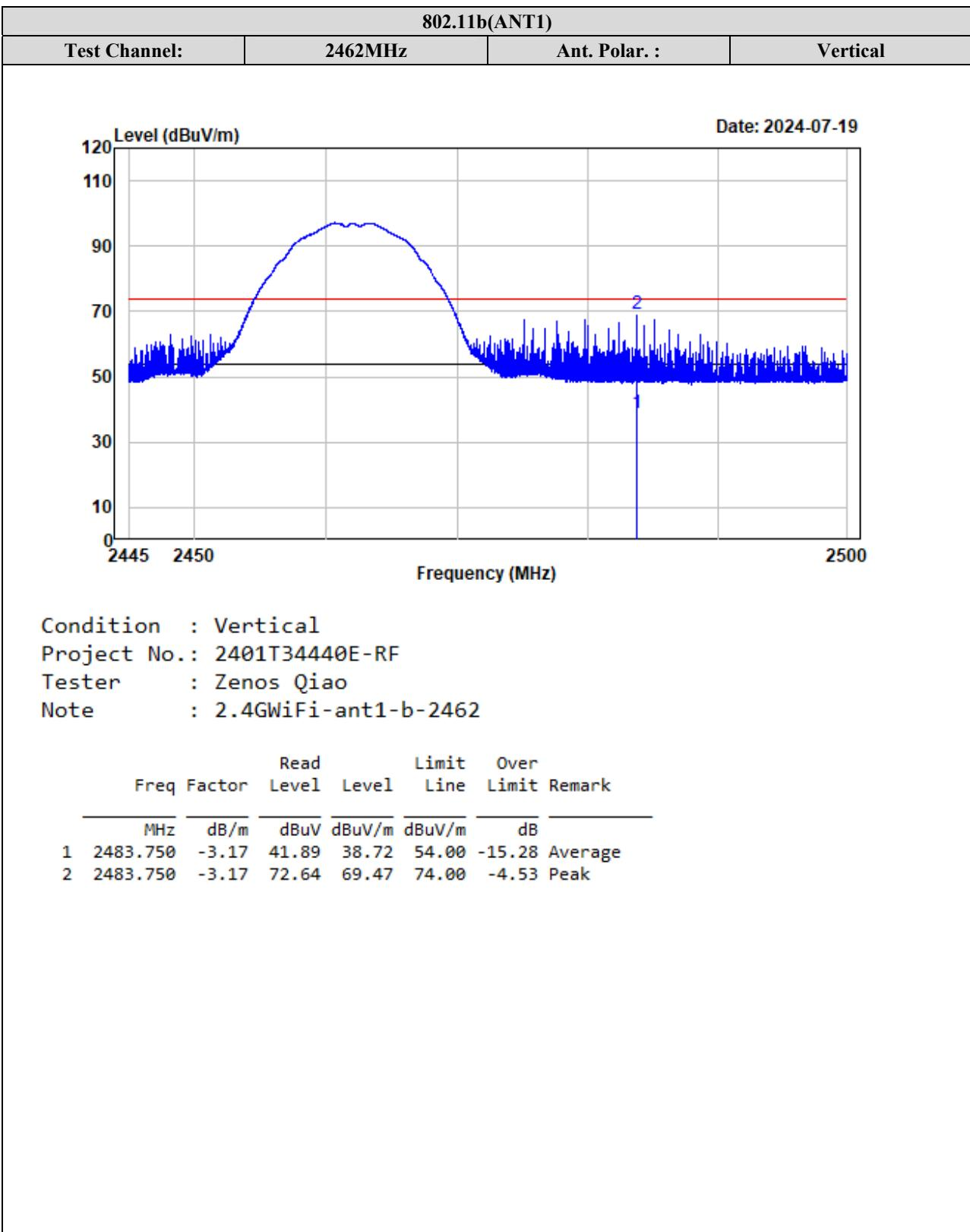
**For Module YL43456****Test plots for Band Edge Measurements (Radiated):**
