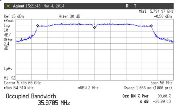
Transmit Freq Error 3.842 kHz x dB Bandwidth 44.381 MHz
