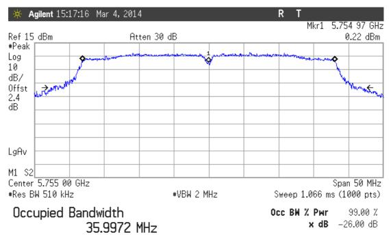
Transmit Freq Error -30.594 kHz x dB Bandwidth 44.074 MHz
