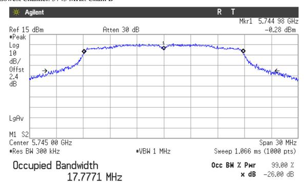
Transmit Freq Error -30.073 kHz x dB Bandwidth 24.412 MHz
