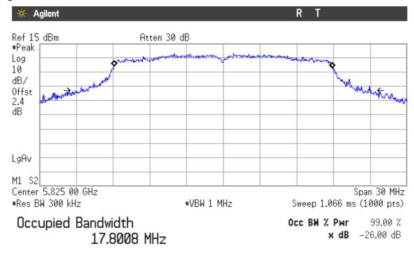
Transmit Freq Error -9.586 kHz x dB Bandwidth 24.072 MHz
