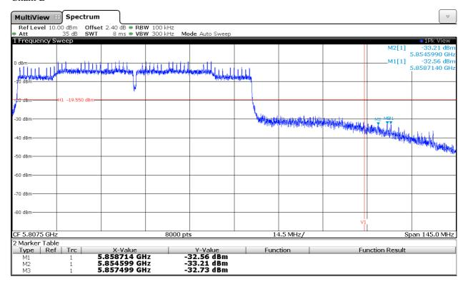
Verdict: PASS (NOTE: The limit is set to -20 dBc since the maximum peak conducted output power was measured for this mode.)
