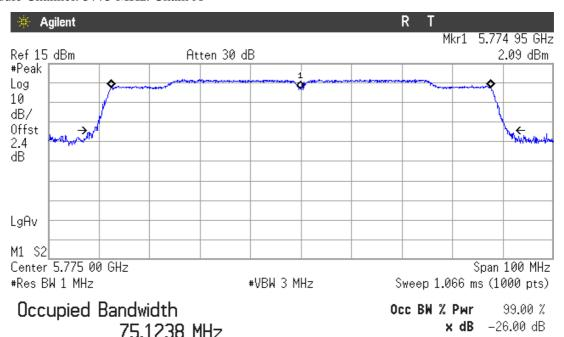
Transmit Freq Error -12.748 kHz x dB Bandwidth 81.829 MHz
