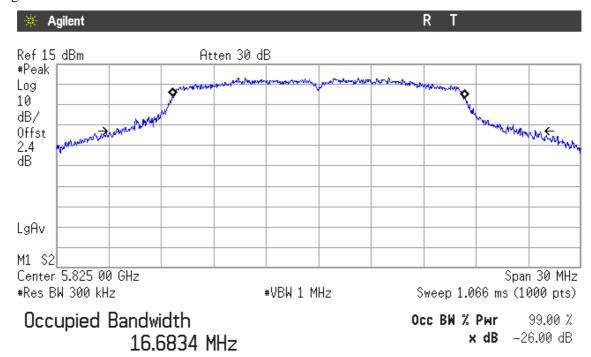
Transmit Freq Error -21.479 kHz x dB Bandwidth 23.958 MHz
