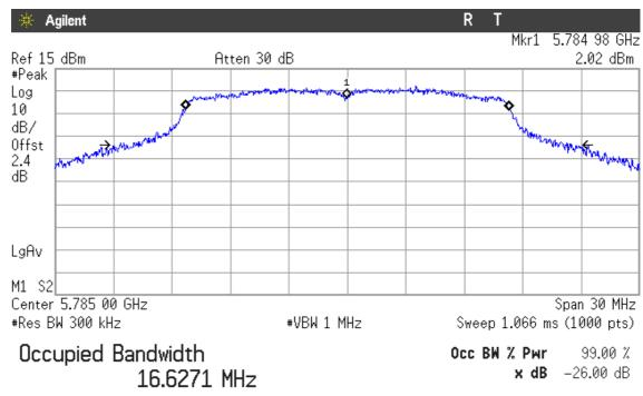
Transmit Freq Error -1.393 kHz x dB Bandwidth 23.250 MHz
