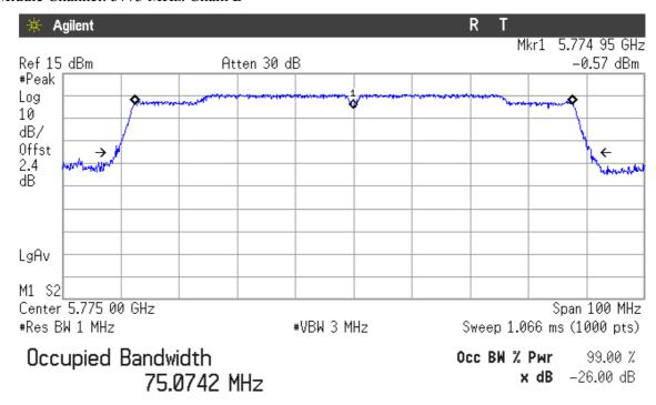
Transmit Freq Error -36.161 kHz x dB Bandwidth 81.659 MHz
