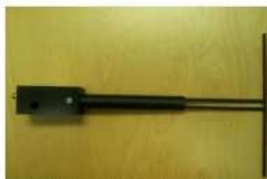
Figure 1 – MVG COMOSAR Validation Dipole
