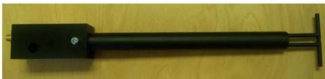
Figure 1 – MVG COMOSAR Validation Dipole
