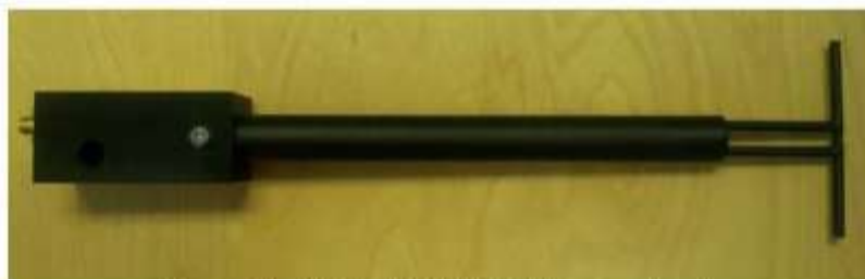
Figure 1 – MVG COMOSAR Validation Dipole
