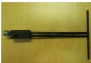
Figure 1 – MVG COMOSAR Validation Dipole
