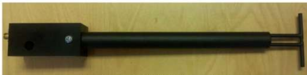
Figure 1 – MVG COMOSAR Validation Dipole
