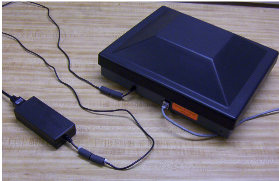
Photograph of ILS Non-contact Programmer 2.0 and Deltron 11985 AC Adapter
