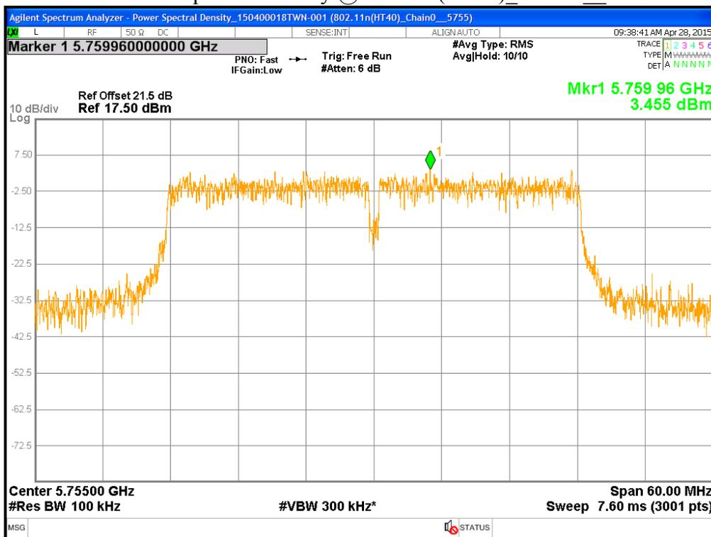
**Chain 0: Power Spectral Density @ 802.11n(HT40)\_Chain0\_5795MHz**
