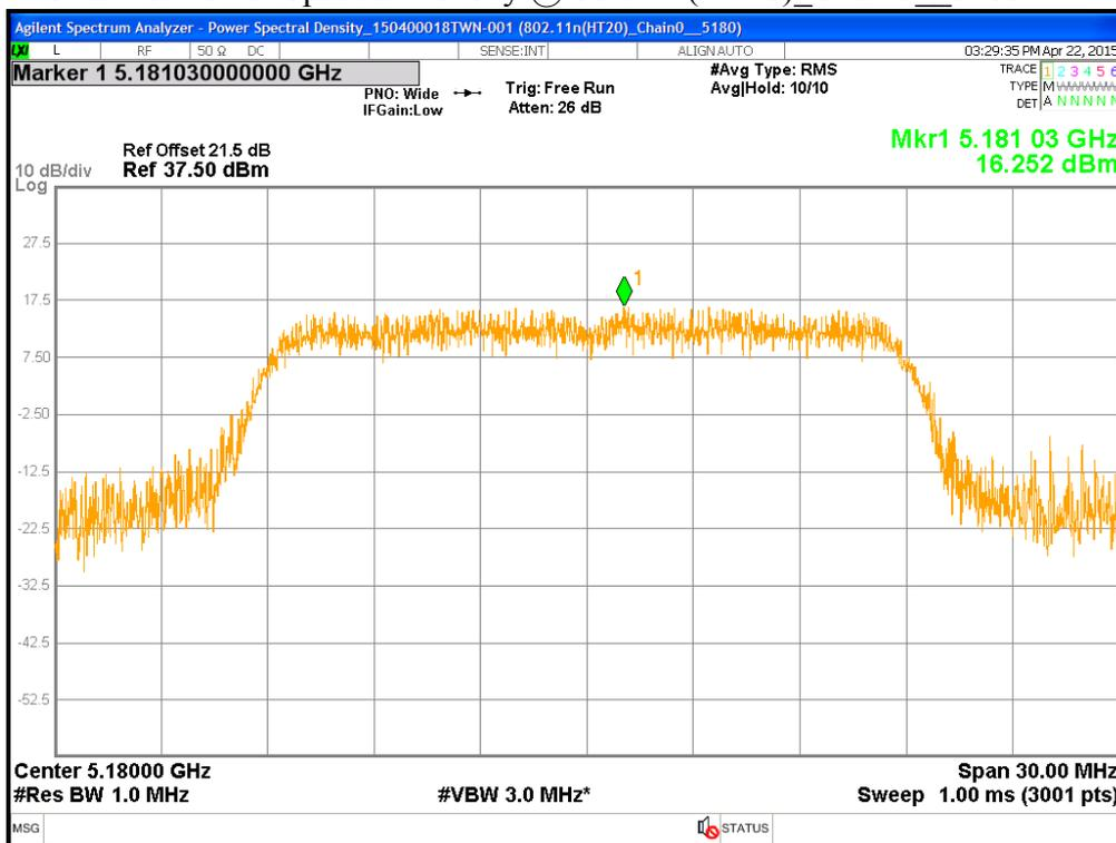
**Chain 0: Power Spectral Density @ 802.11n(HT20)\_Chain0\_5200MHz**
