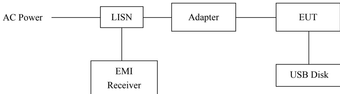
**Note:** The EUT was tested while in normal communication mode.
