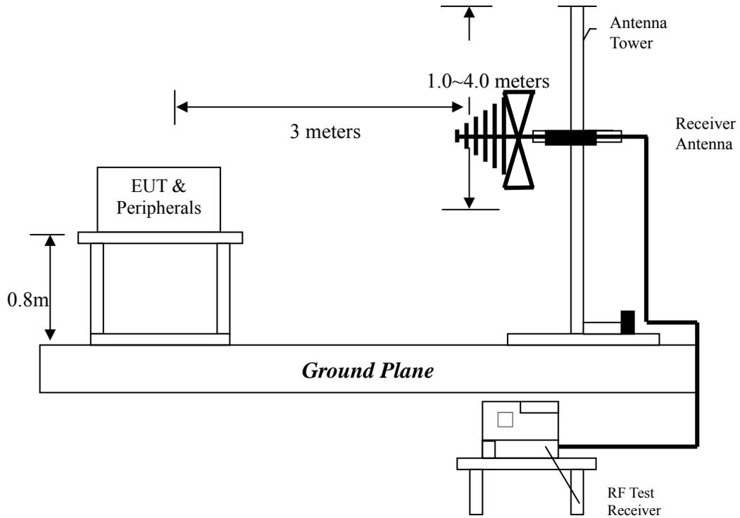
**6.5.3 Radiated emission above 1GHz using Horn Antenna**
