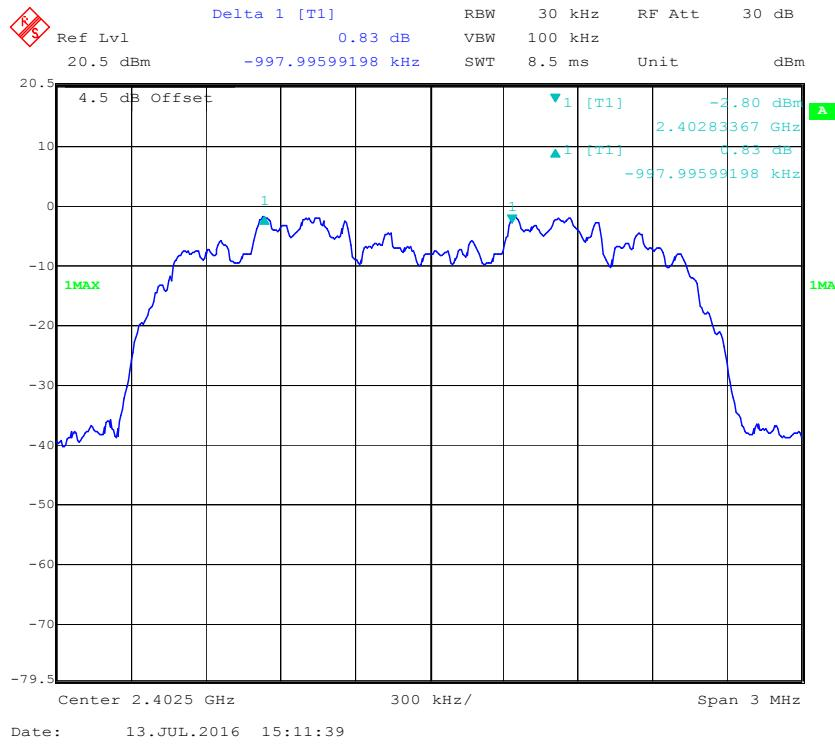
**EDR ( $\pi/4$ -DQPSK): Middle Channel**
