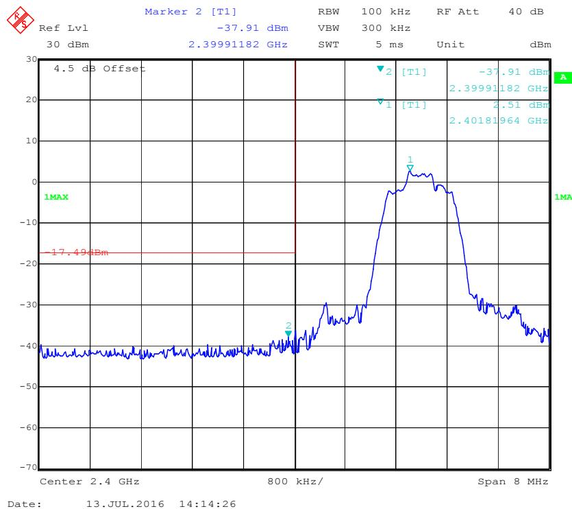
**BDR (GFSK): Band Edge-Right Side**
