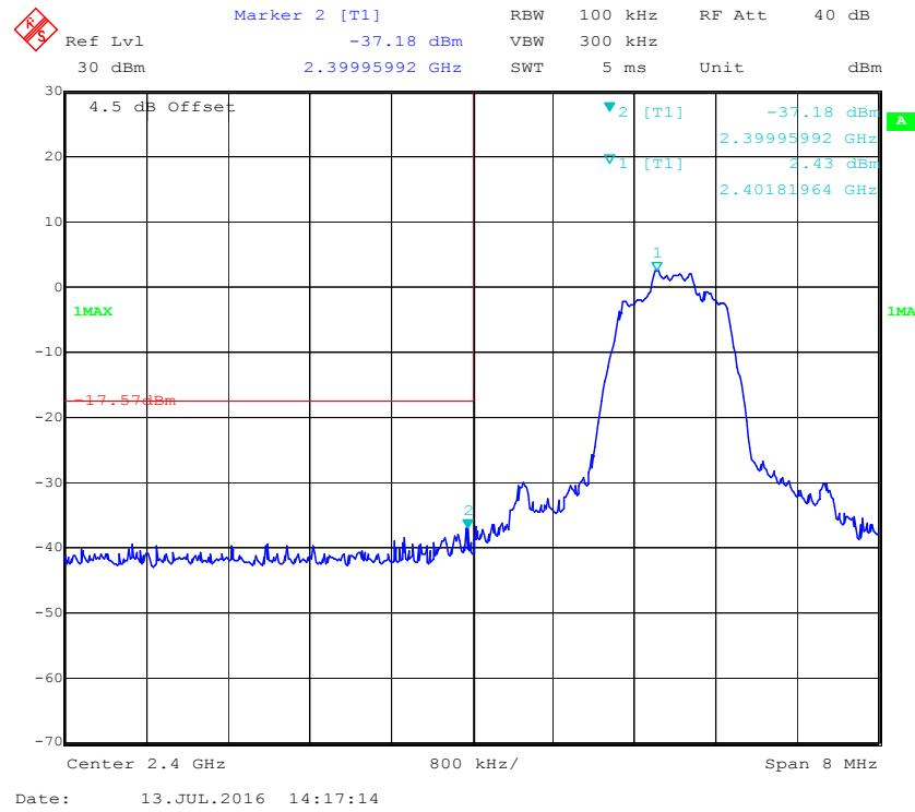
**EDR ( $\pi/4$ -DQPSK): Band Edge-Right Side**
