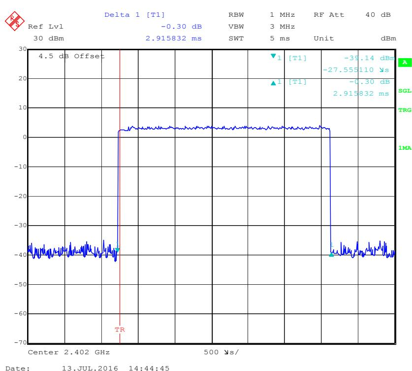
**Pulse time, Middle Channel, 2DH5**
