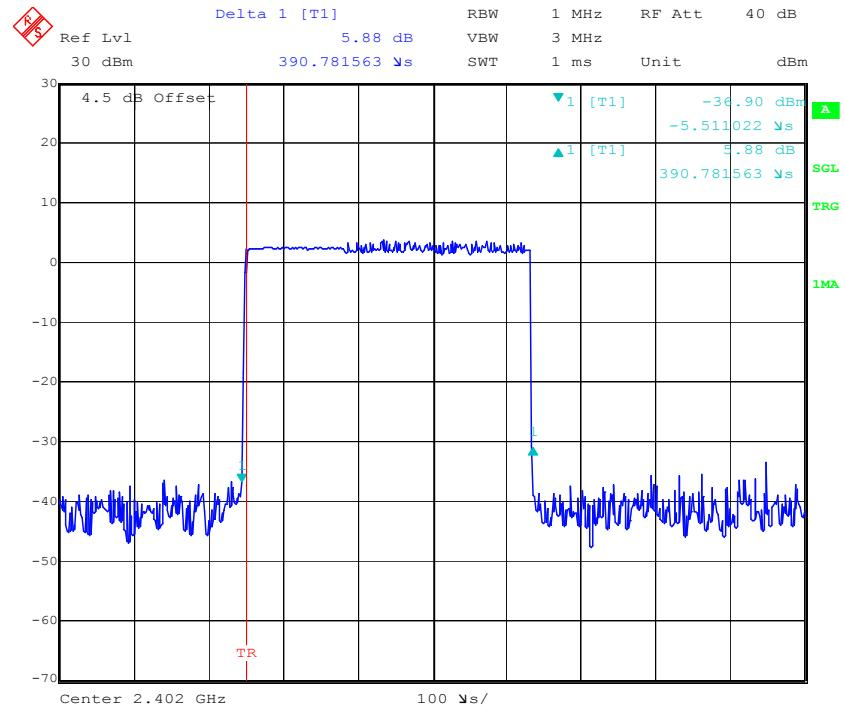
**Pulse time, Middle Channel, 2DH1**
