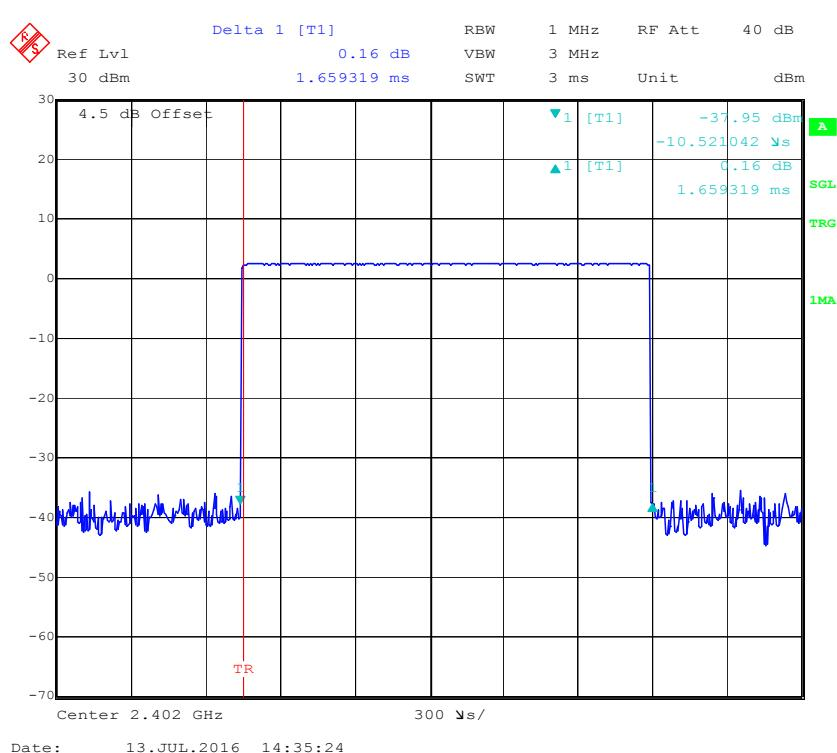
**Pulse time, Middle Channel, DH3**
