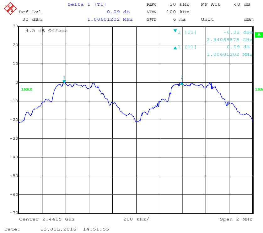
**BDR (GFSK): High Channel**
