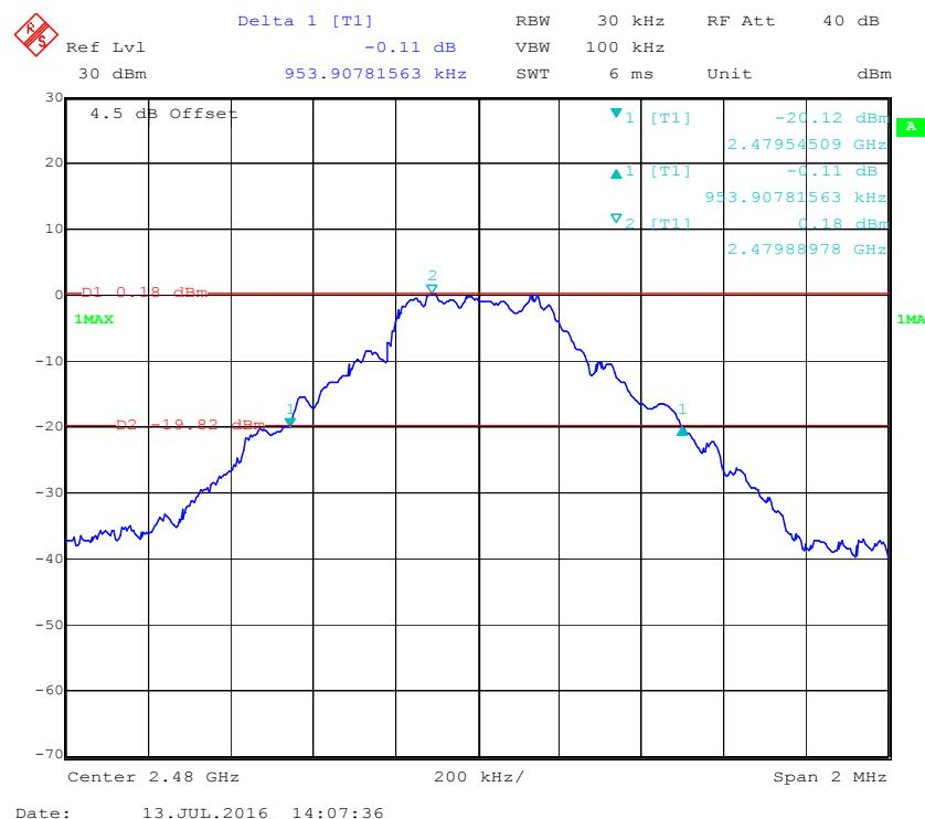
**EDR ( $\pi/4$ -DQPSK): Low Channel**
