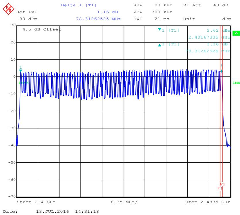
**EDR ( $\pi/4$ -DQPSK): Number of Hopping Channels**
