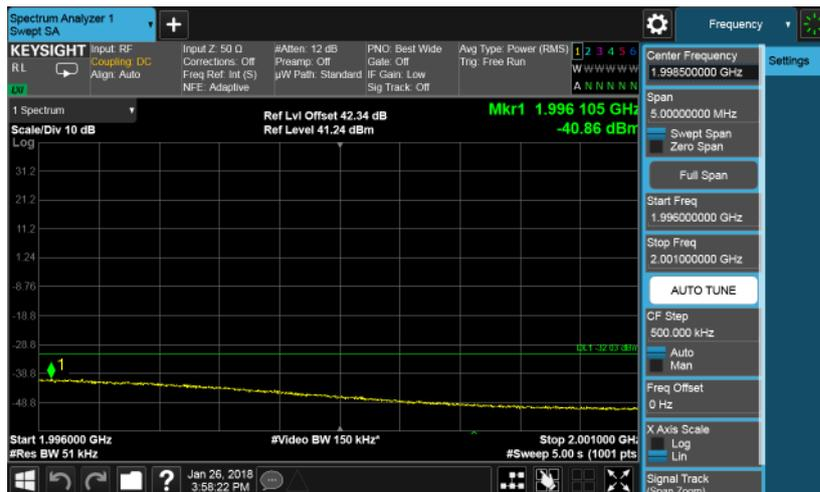
Configuration WCDMA+LTE-MIMO-MC-4-BE (2WCDMA, 16QAM + 1LTE, QPSK)
