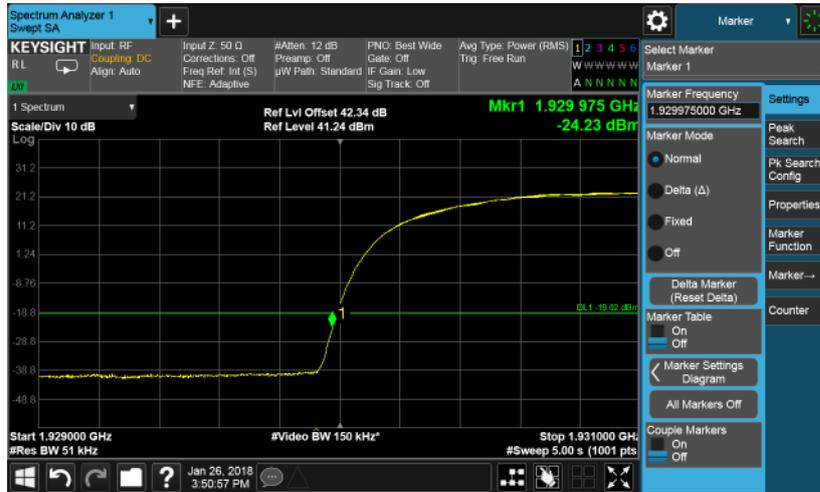
The channel power of 50.0KHz for 1929.975MHz is -28.67dBm, which is within the limit of -19.02dBm.
