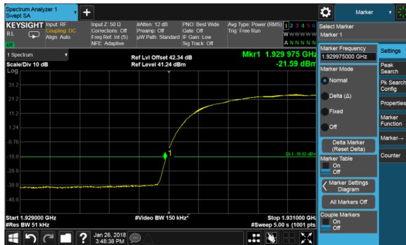
The channel power of 50.0KHz for 1929.975MHz is -27.87dBm, which is within the limit of -19.02dBm.
