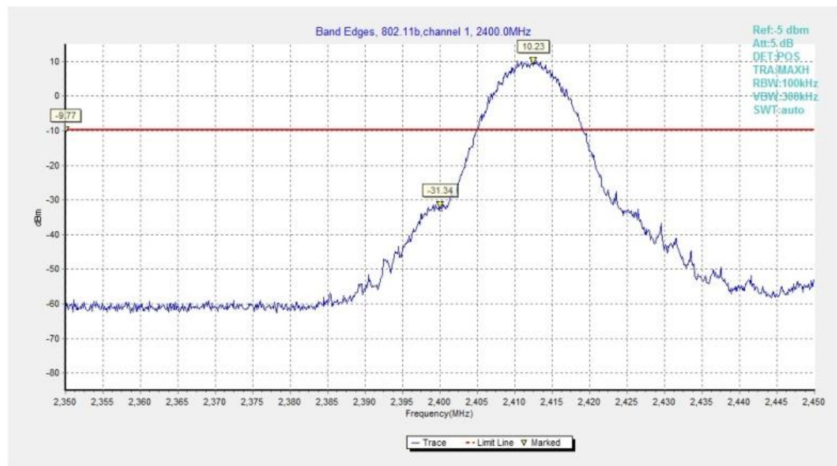
Fig.A.5.1 Band Edges (802.11b, Ch 1)
