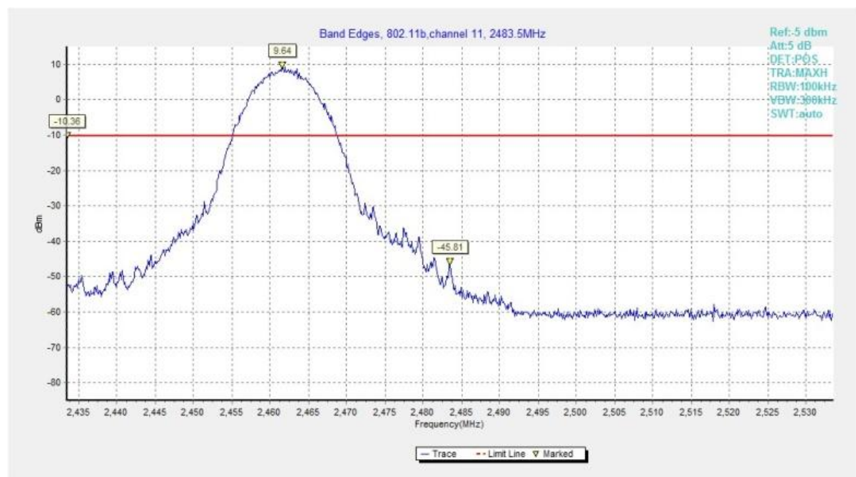
Fig.A.5.2 Band Edges (802.11b, Ch 11)
