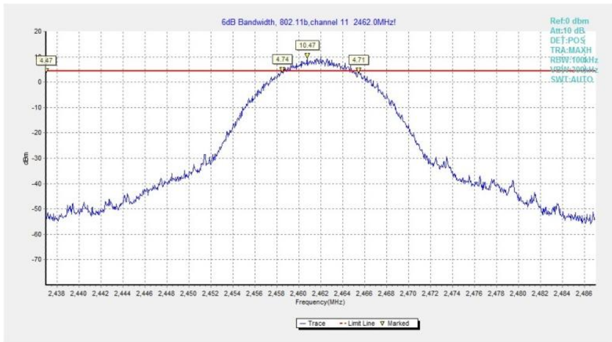
Fig.A.4.3 Occupied 6dB Bandwidth (802.11b, Ch 11)
