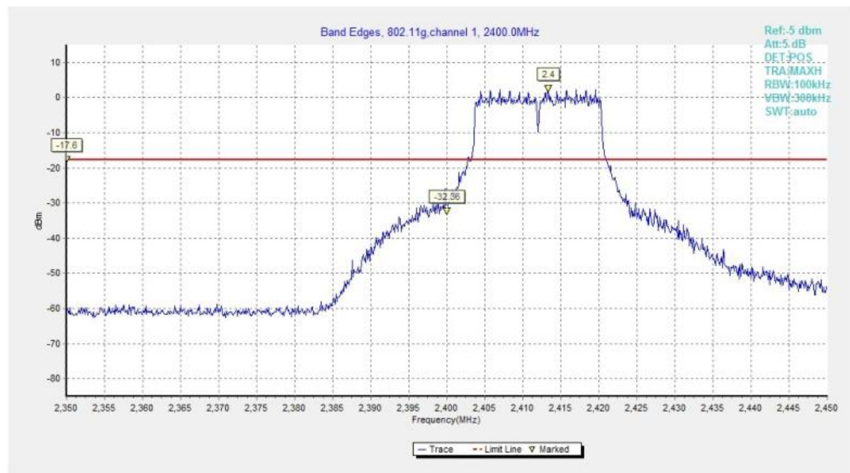
Fig.A.5.3 Band Edges (802.11g, Ch 1)
