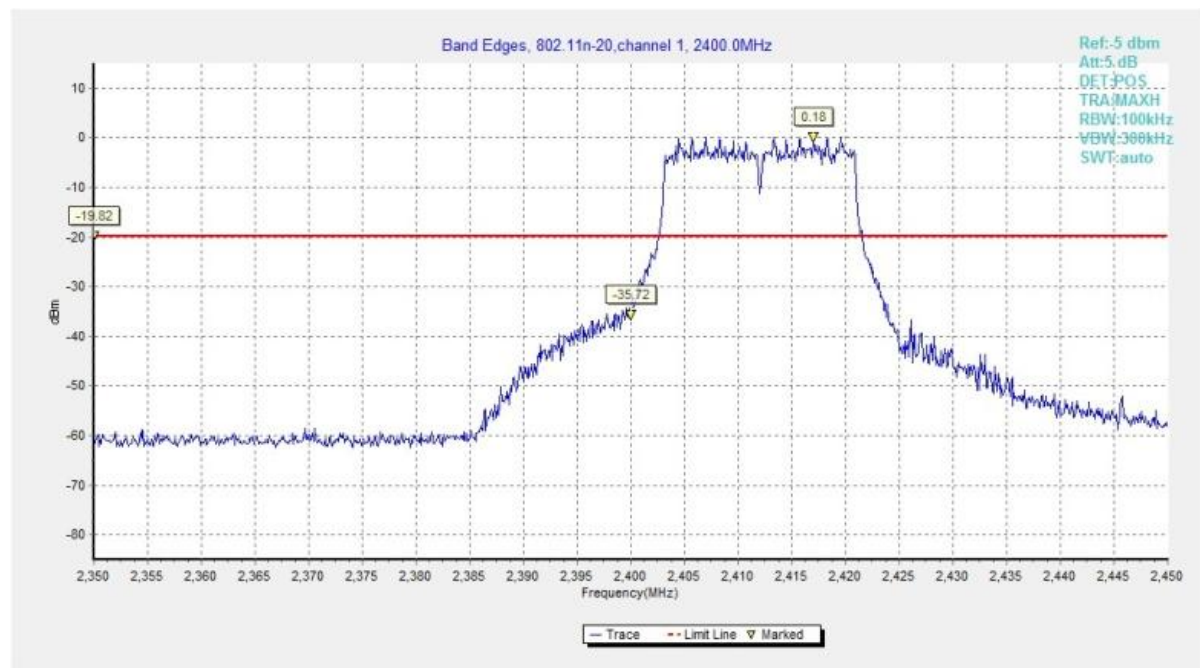
Fig.A.5.5 Band Edges (802.11n-HT20, Ch 1)
