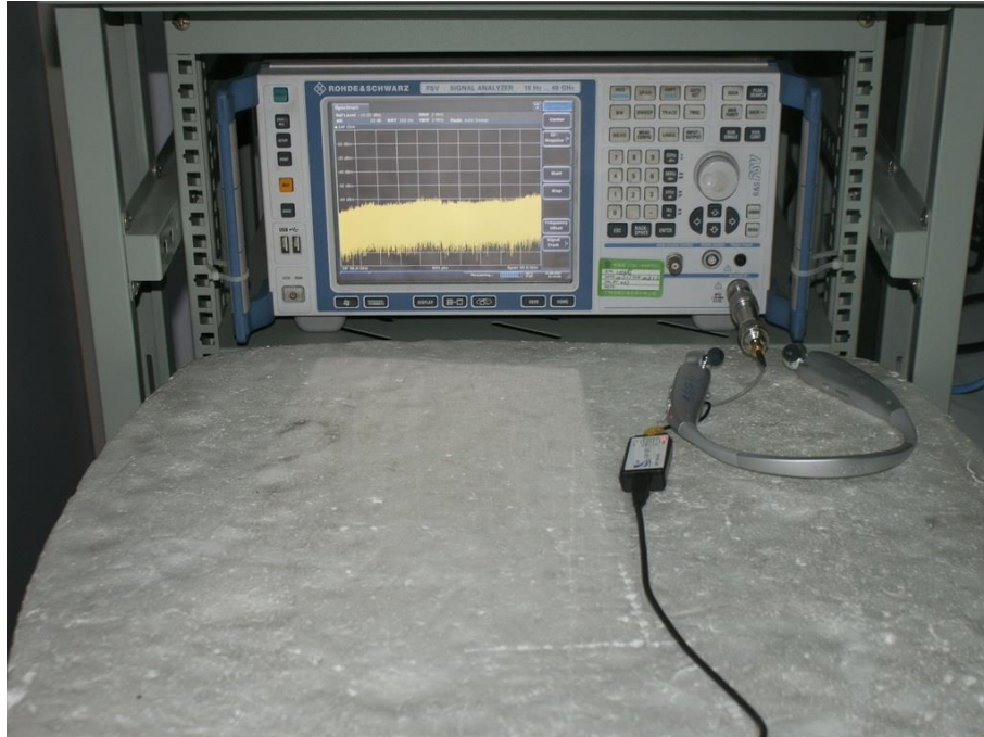
Photograph 2: Set-up for Spurious Emissions (9kHz-30MHz)
