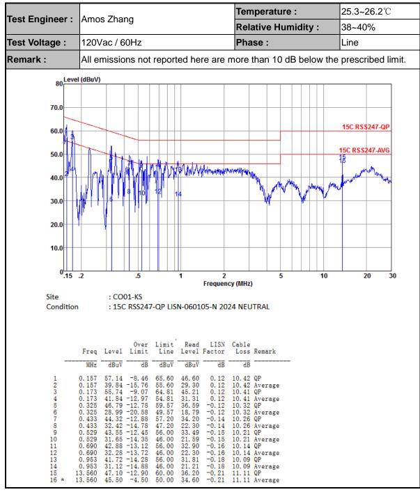
Remark: 13.560MHz is the NFC RF fundamental signal.
