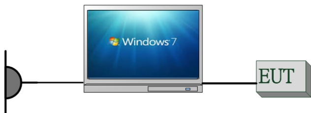
Fig. 2-2 AC Power Line Conducted Emission
