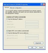
Go back to Internet Protocol (TCP/IP) and double click →tick "Obtain an IP address automatically" and "Obtain DNS server address automatically".
