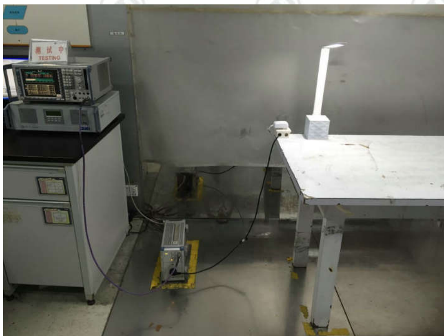
Conducted emissions Test Setup
