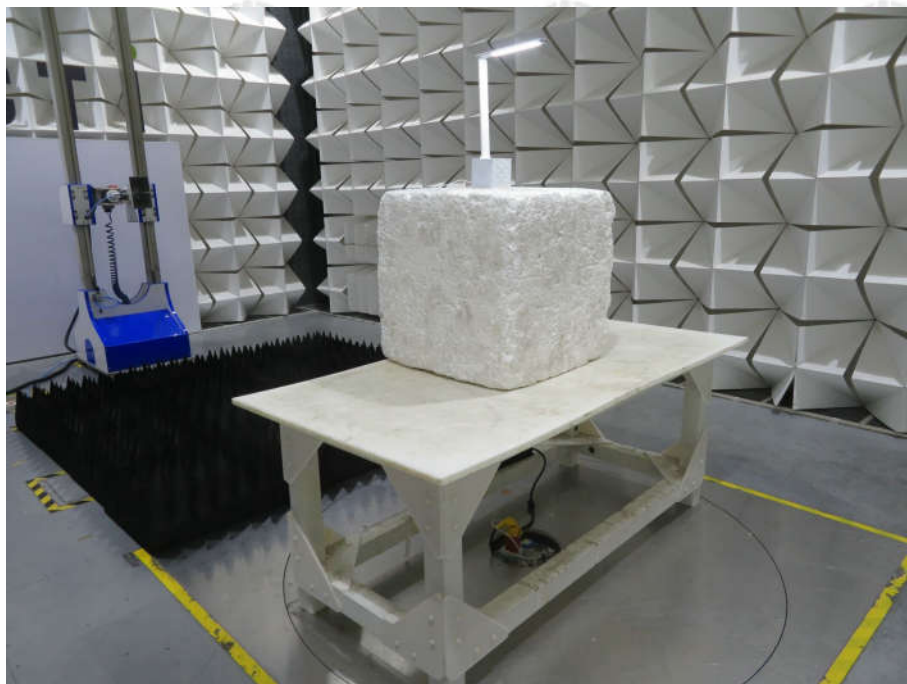
Radiated spurious emission Test Setup-3(Above 1GHz)
