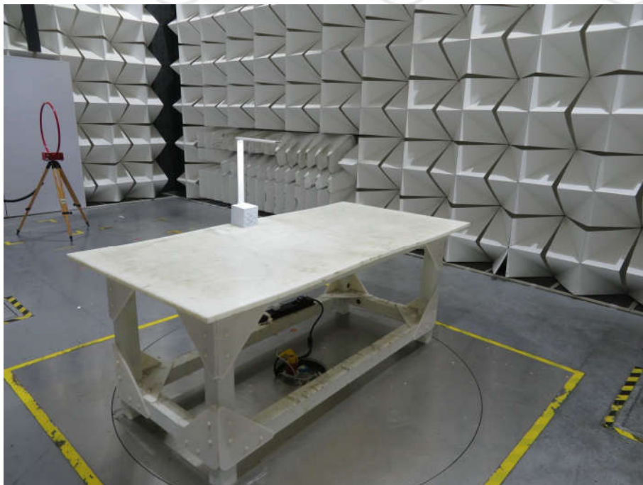
Radiated spurious emission Test Setup-1(Below 30M)
