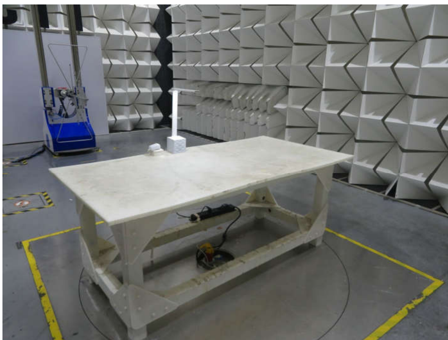
Radiated spurious emission Test Setup-2(Below 1GHz)
