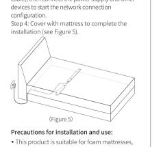
spring mattresses, latex mattresses with the thickness of 6-30 cm. The use of water beds, air mattresses, and high-hardness mattresses may cause lower monitoring accuracy or function failure The single bed version and the single bed extended version are only suitable for single person usage, and the double bed version is
