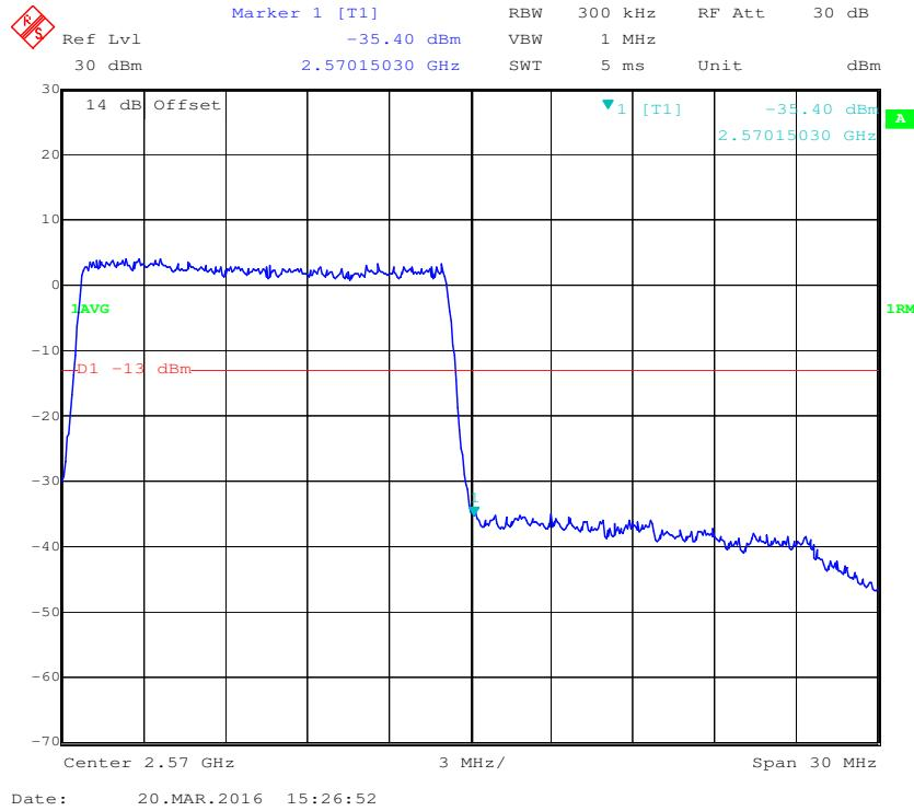
**QPSK (20 MHz, FULL RB) - Left Band Edge**
