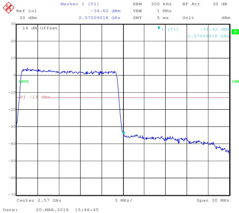
**16-QAM (15 MHz, FULL RB) - Left Band Edge**
