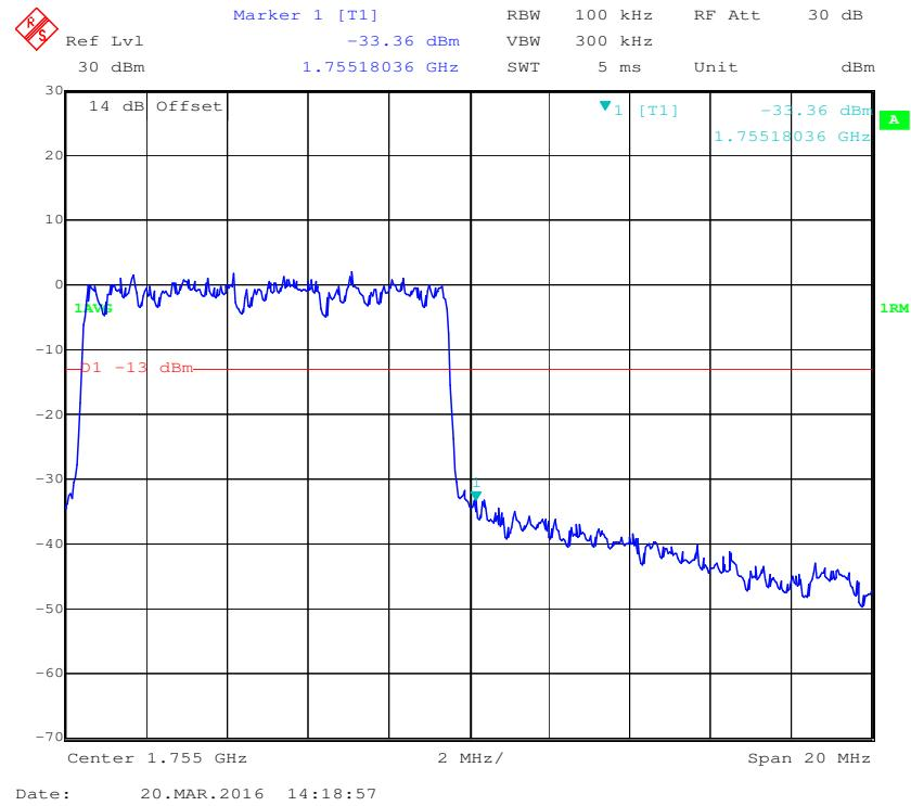
**QPSK (15.0 MHz, FULL RB) - Left Band Edge**
