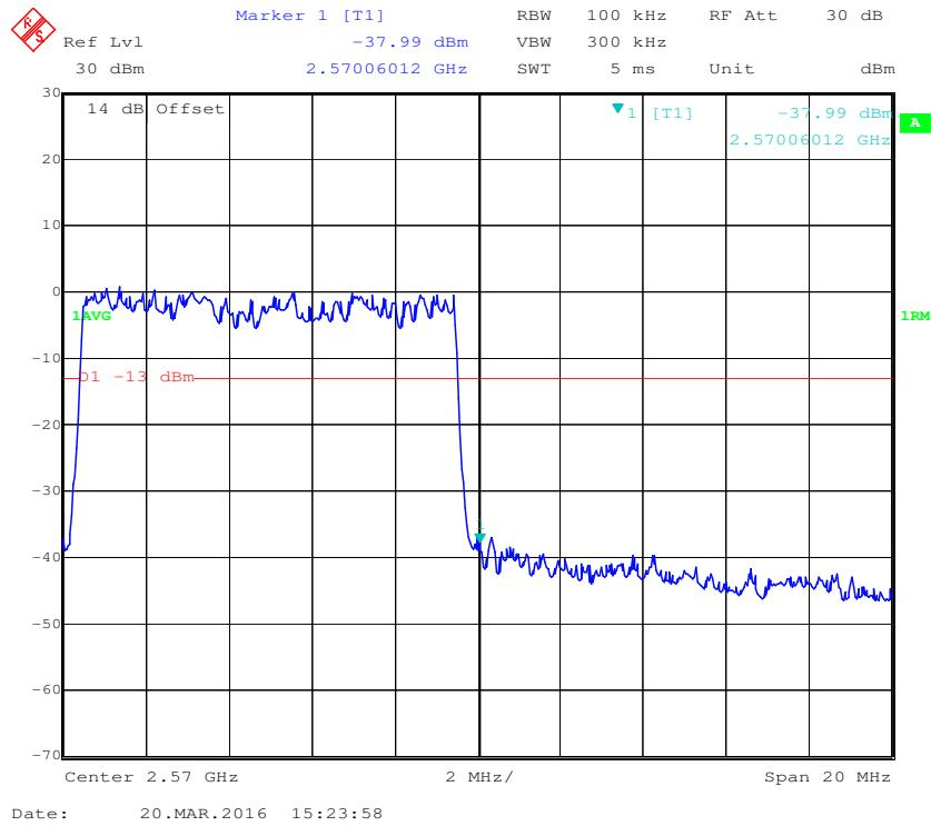
**QPSK (15 MHz, FULL RB) - Left Band Edge**
