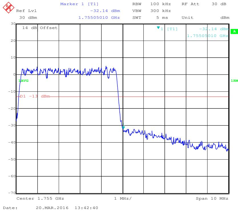
**16-QAM (5.0 MHz, FULL RB) - Left Band Edge**
