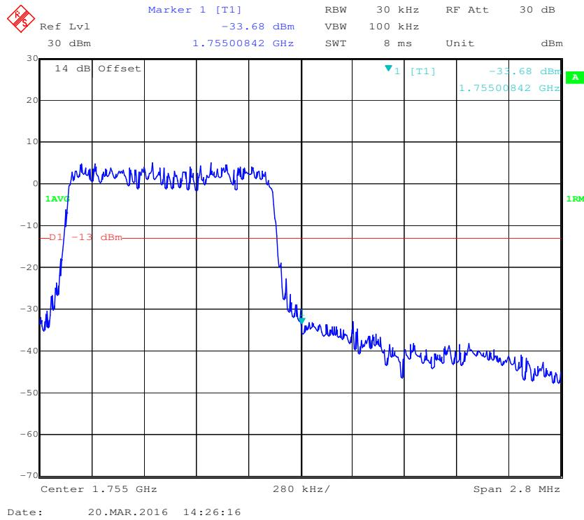
**QPSK (3.0 MHz, FULL RB) - Left Band Edge**
