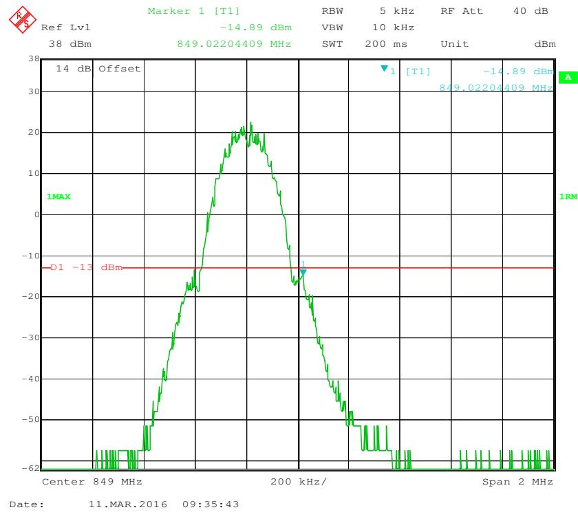
**Cellular Band, Left Band Edge for EGPRS Mode**
