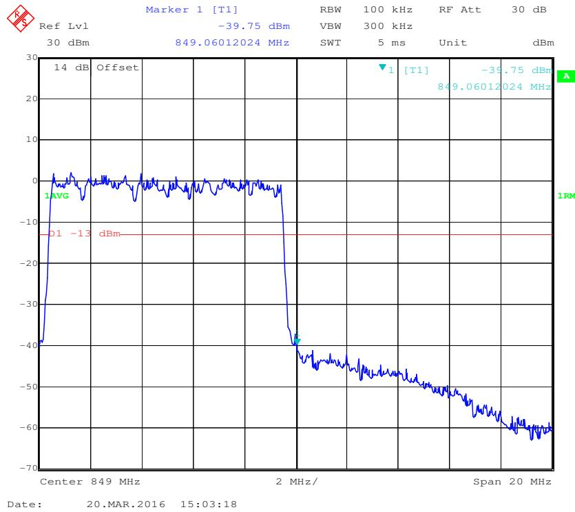
**16-QAM (10.0 MHz, FULL RB) - Left Band Edge**
