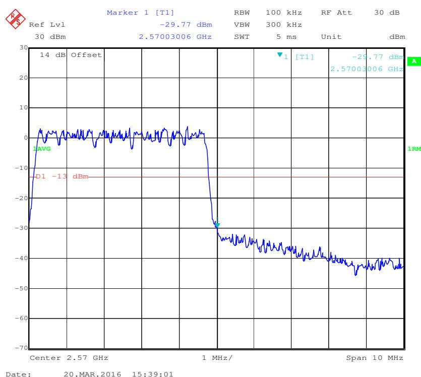
**16-QAM (5.0 MHz, FULL RB) - Left Band Edge**
