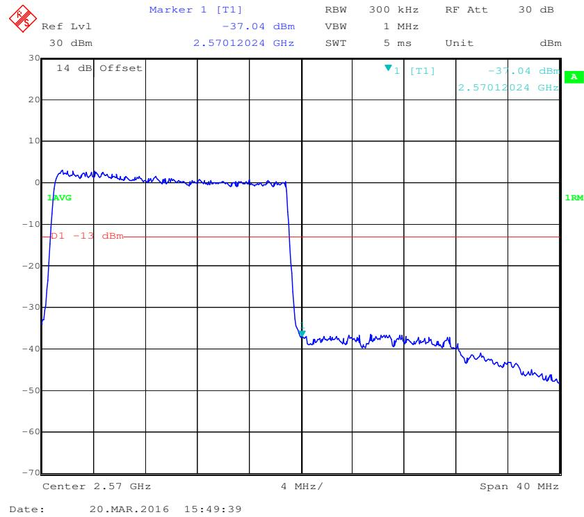
**16-QAM (20 MHz, FULL RB) - Left Band Edge**
