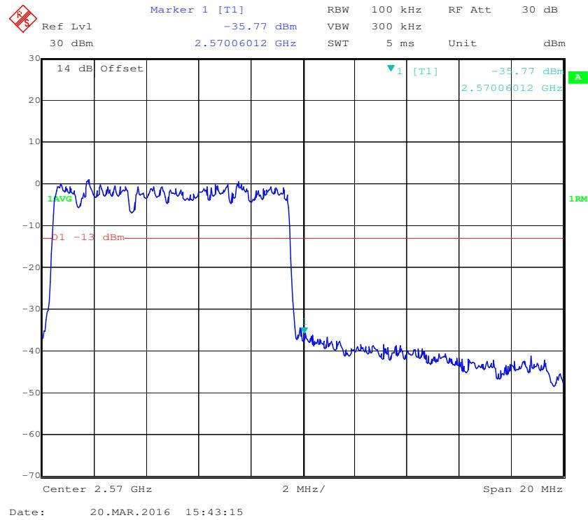
**16-QAM (10.0 MHz, FULL RB) - Left Band Edge**
