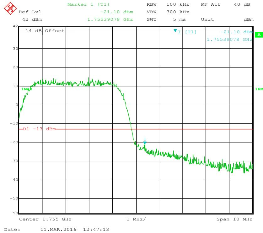
**AWS Band, Left Band Edge for HSUPA (BPSK) Mode**
