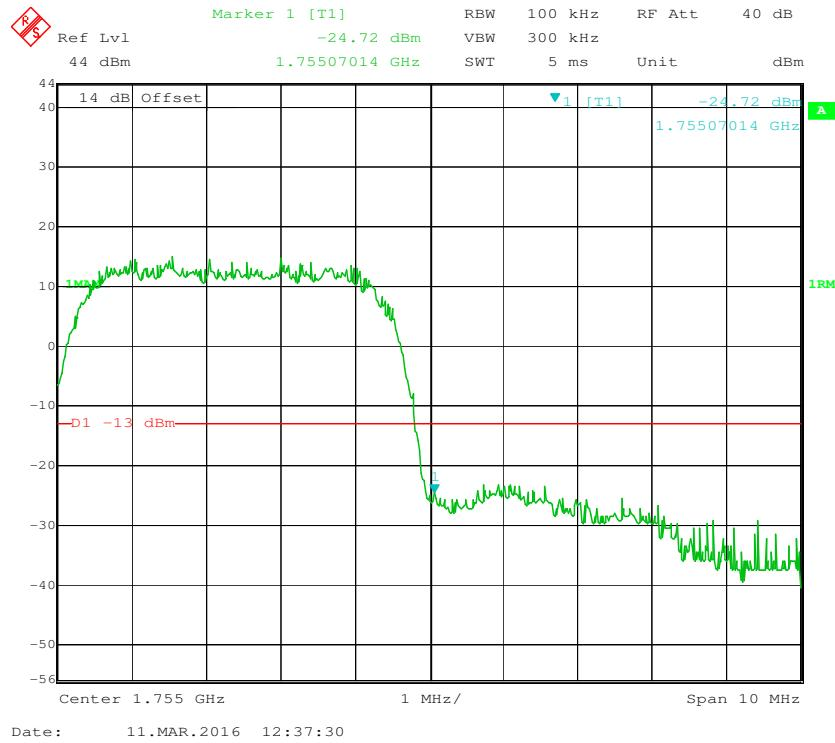
**AWS Band, Left Band Edge for HSDPA (16QAM) Mode**
