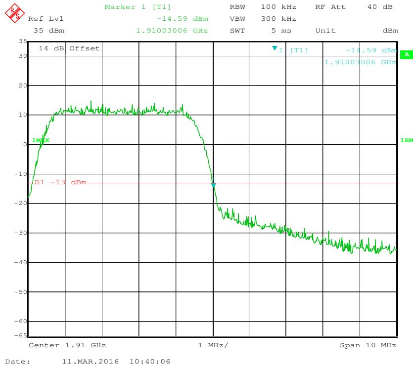
**AWS Band, Left Band Edge for RMC (BPSK) Mode**
