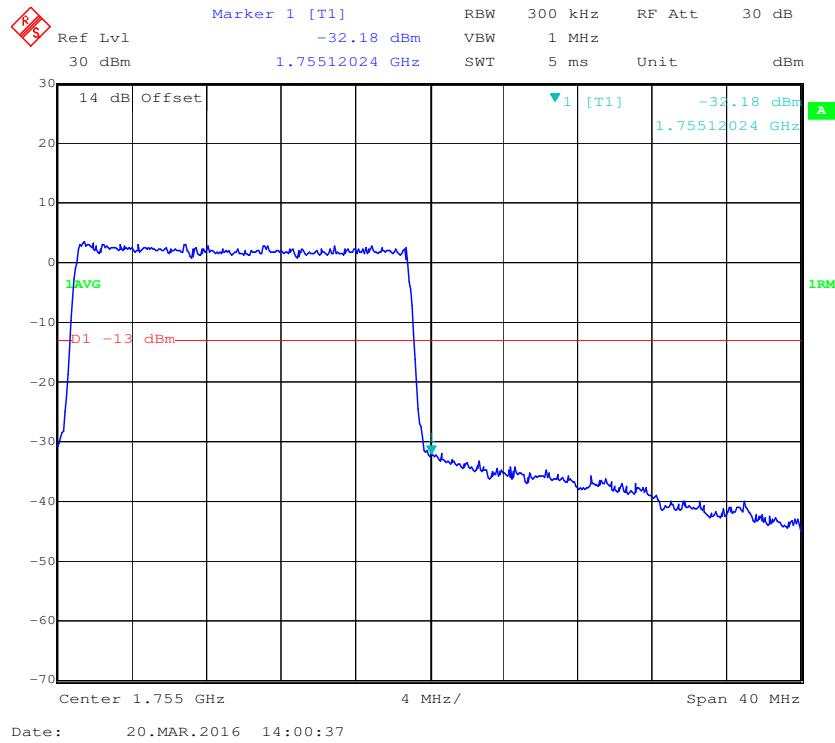
**16-QAM (20.0 MHz, FULL RB) - Left Band Edge**
