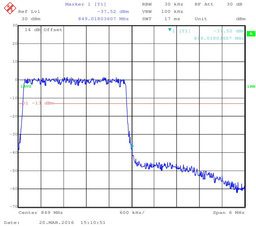
**QPSK (5.0 MHz, FULL RB) - Left Band Edge**
