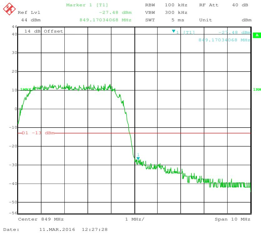
**PCS Band, Left Band Edge for GSM (GMSK) Mode**
