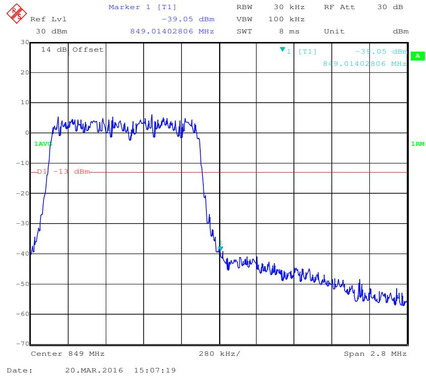
**QPSK (3.0 MHz, FULL RB) - Left Band Edge**
