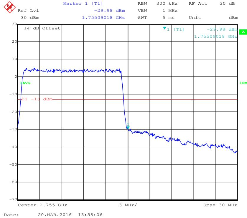
**16-QAM (15.0 MHz, FULL RB) - Left Band Edge**
