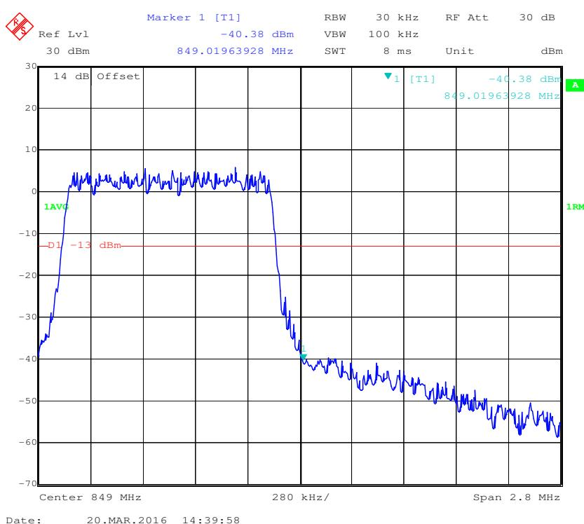
**16-QAM (1.4 MHz, FULL RB) - Left Band Edge**
