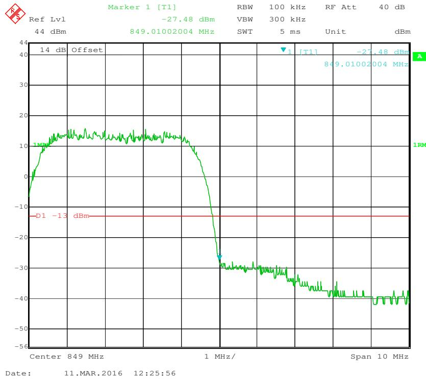
**Cellular Band, Left Band Edge for HSDPA (16QAM) Mode**
