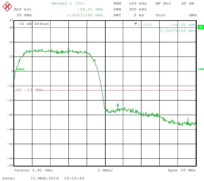
**PCS Band, Left Band Edge for HSDPA (16QAM) Mode**
