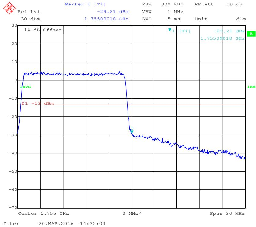
**QPSK (20.0 MHz, FULL RB) - Left Band Edge**
