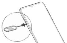
2. Pull out the card tray and place the nano-SIM card and the microSDXC card (optional) on the tray, as shown. Carefully slide the tray back into place.
