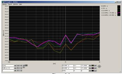
Figure 8-3 UMTS Audio Band Magnetic Noise
