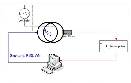
Figure 4-1 Validation Setup with Helmholtz Coil
