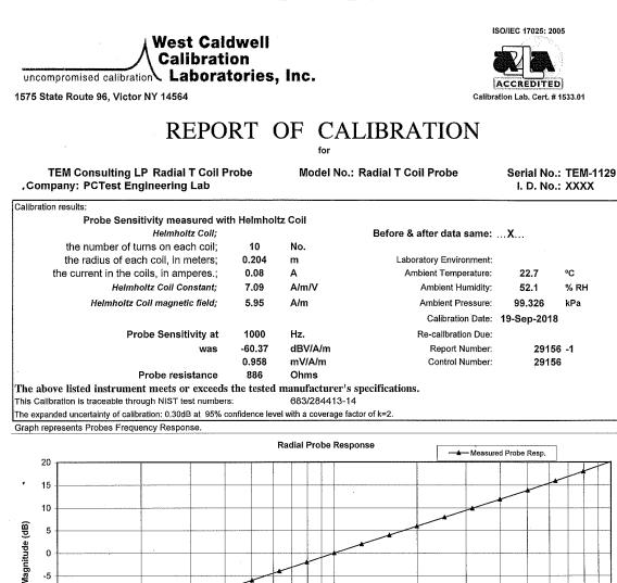
The above listed instrument was checked using calibration procedure documented in West Caldwell
