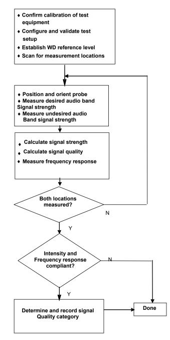
Figure 4-14 C63.19 T-Coil Signal Test Process
