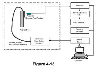
Audio Magnetic Field Test Setup
