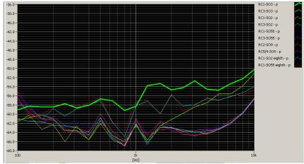
Figure 8-1 CDMA Audio Band Magnetic Noise
