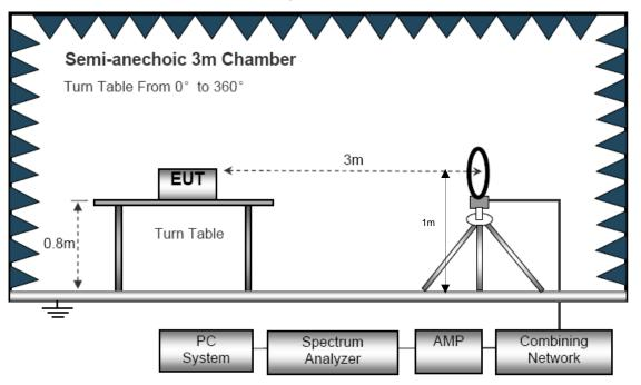
(B) Radiated Emission Test-Up Frequency 30MHz~1GHz
