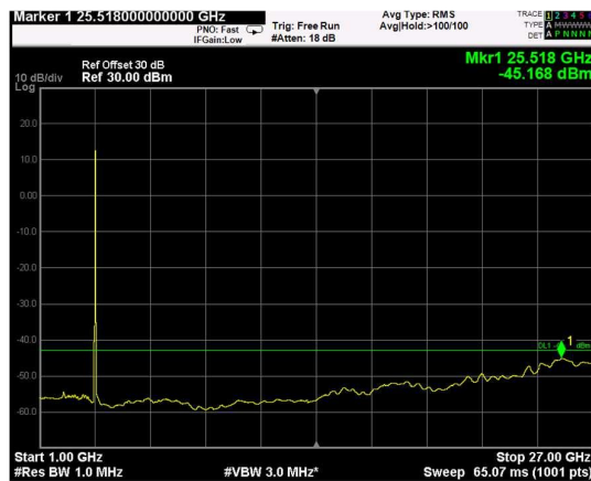
Channel: BOTTOM, Modulation: 64QAM, BW=15MHz, Range: 1GHz - 27GHz
