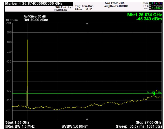
Channel: BOTTOM, Modulation: QPSK, BW=20MHz, Range: 1GHz - 27GHz
