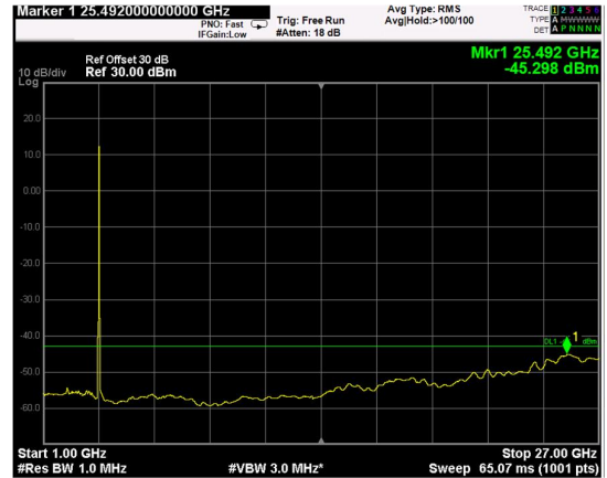
Channel: BOTTOM, Modulation: 16QAM, BW=15MHz, Range: 1GHz - 27GHz
