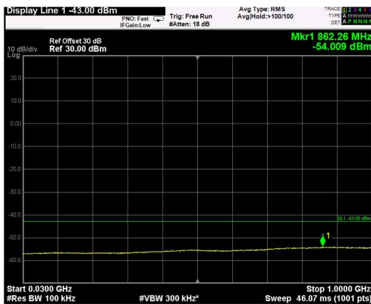
Channel: BOTTOM, Modulation: 64QAM, BW=15MHz, Range: 30MHz - 1GHz
