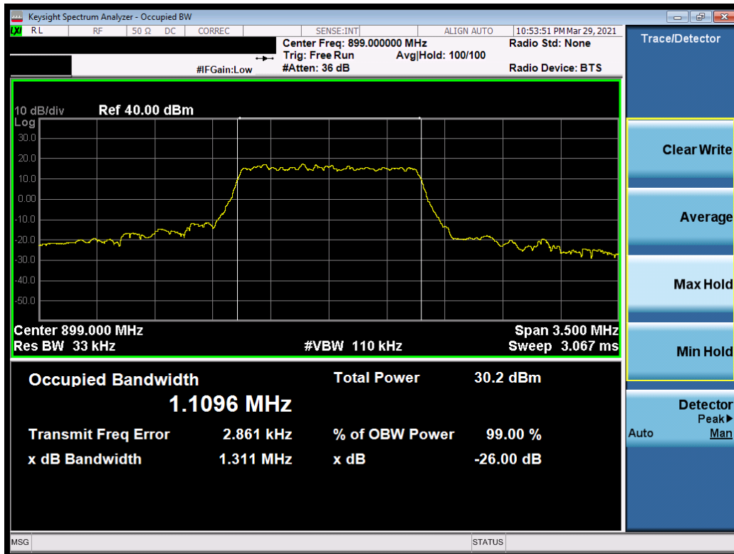
Plot 7-7. Occupied Bandwidth Plot (1.4MHz, QPSK, RB 6, RB Offset 0, NB=0)
