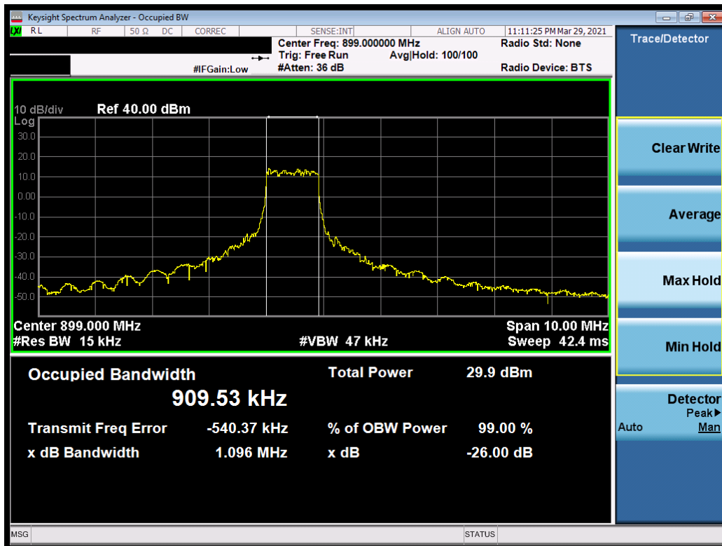
Plot 7-5. Occupied Bandwidth Plot (3MHz, 16-QAM, RB 5, RB Offset 1, NB=0)
